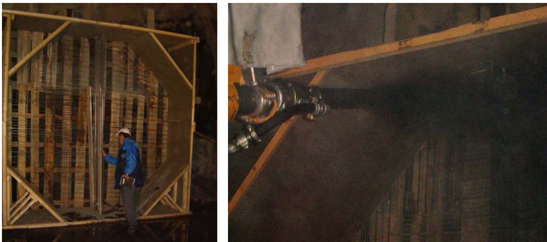
Figure 11: Spraying trial on panel reproducing conditions at Grimsel
