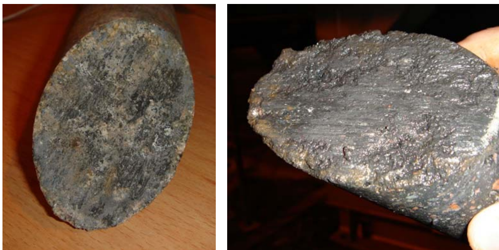
Figure 25: Detail of inclined from the top of the plug; rock core (left) and concrete core (right) both with slickensides
