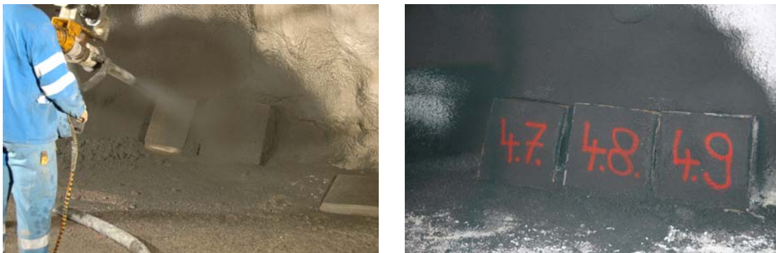
Figure 27: Pre-tests on panels (700 mm x 700 mm) using mix 4 and different dosage of set accelerator.
