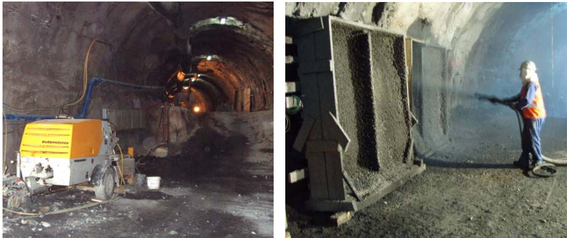
Figure 8: Spraying trial on panel reproducing conditions at Äspö HRL
