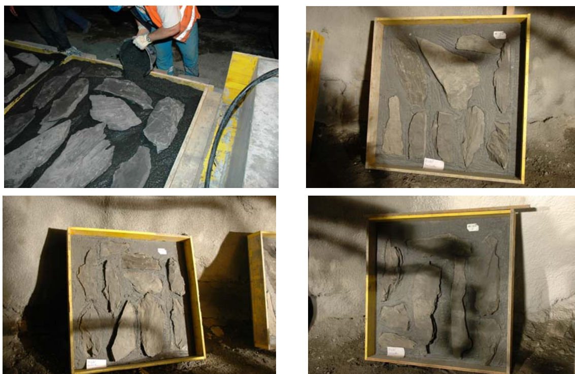
Figure 28: Preparation of Opalinus Clay test panels (1.5 m x 1.5 m).
