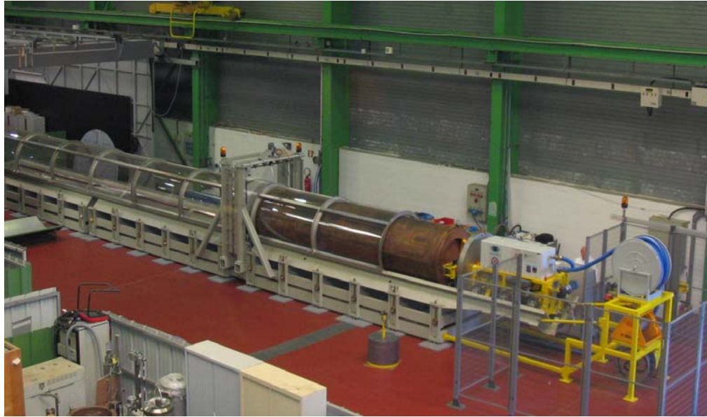
Figure 15: ANDRA Deposition Equipment Test Bench
