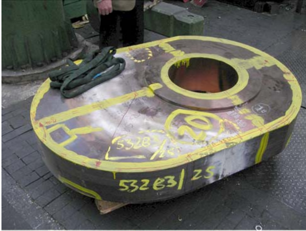
Figure 10: Fabrication of borehole lock
