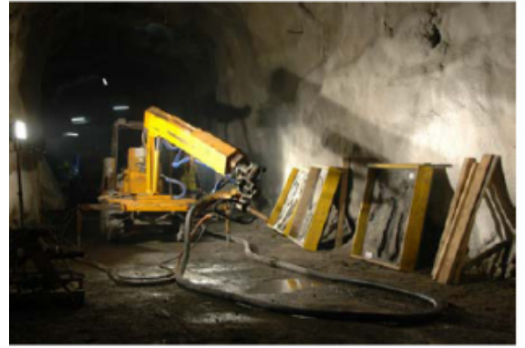
Figure 21: Pilot tests with low-pH shotcrete at the Test Gallery Hagerbach Ltd, Switzerland
