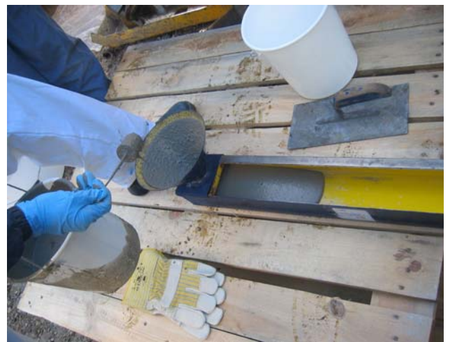
Figure 3: Grout preparation pre-test (check fluidity)
