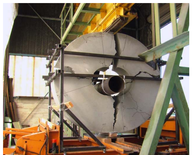
Figure 5: Brazilian Shearing Test
