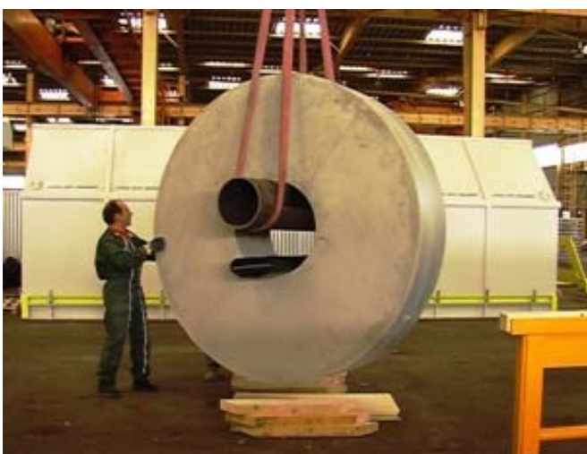
Figure 4: Lifting Test by Ring Central Hole
