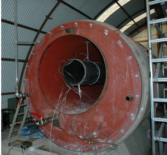
Figure 4: Ondraf/Euridice – Mock-up for backfilling with grout
