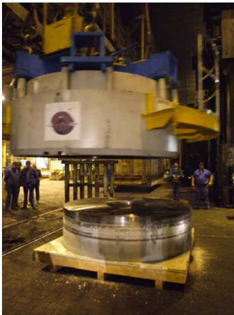
Figure 2: Andra - View of Bentonite Ring just after stripping operation (Dec 2006)
