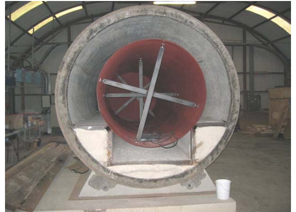
Figure 5: Ondraf/Euridice – Mock-up for backfilling with granular material
