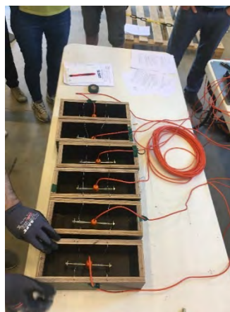
Figure 12: Vibrating wire gage inside wood mould.
