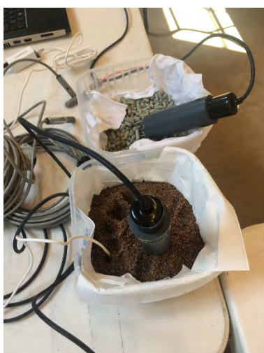
Figure 17: Humidity sensors measuring in different materials (sand and bentonite pellets).
