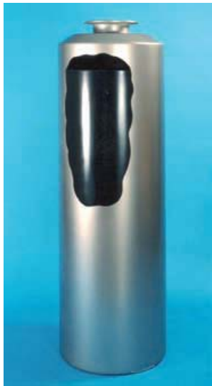
Liquid HLW is solidified into glass blocks inside a stainless steel container like that shown in this cutaway picture. The container is about 1.3 m tall.
