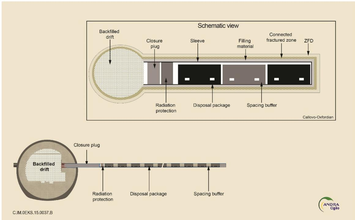
**Figure 2.1:** Illustration of the HLW disposal cell design. ZFD is the French acronym for the discrete fracture zone, part of the excavation damage zone. From Farrow *et al.* (2019).
