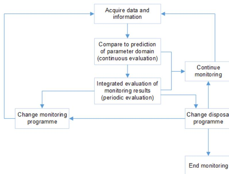
Figure 2.8: Workflow for responding to monitoring results. From White *et al.* (2019).
