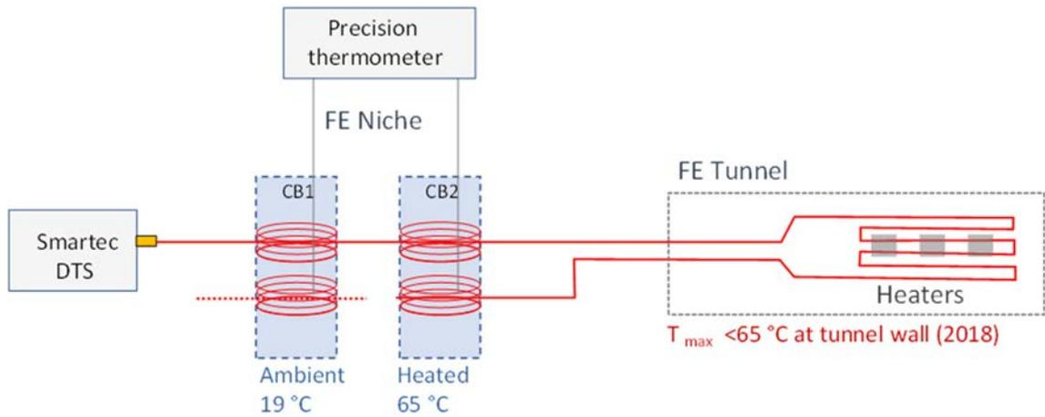
**Figure 4.21:** Single-ended configuration of the dynamic calibration system for DTS units. From Fisch *et al.* (2019).
