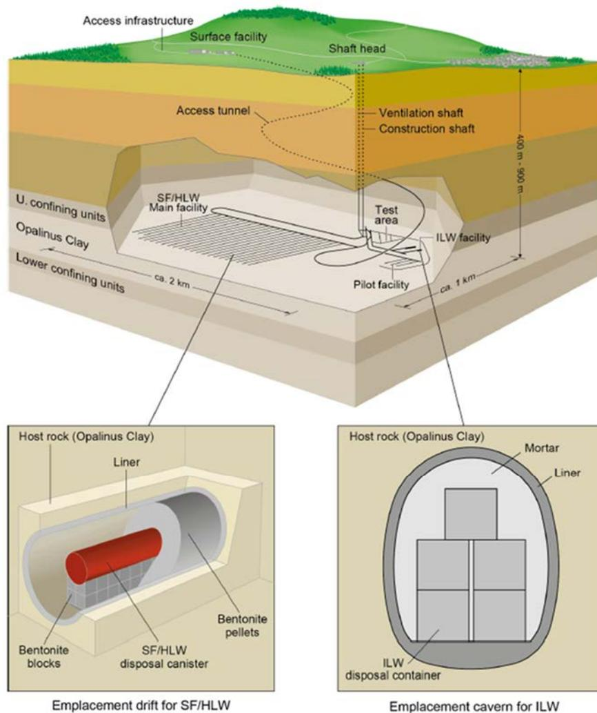
**Figure 2.3:** Possible layout for a deep geological repository for spent fuel, HLW and long-lived ILW in the Opalinus Clay, Switzerland. From Nagra (2016).
