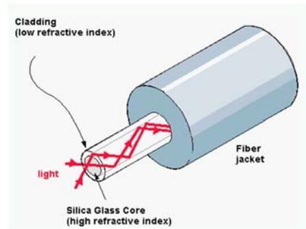
Structure of an optical fibre.
