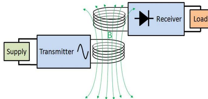
*Wireless power transfer between two coils through electromagnetic induction. The magnetic field produced by current in the transmitter coil is denoted by "B".*
