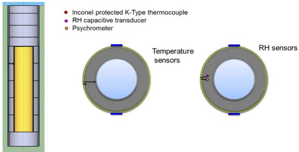
**Figure 4.7:** The location of temperature sensors and relative humidity sensors in the buffer. From VTT *et al.* (2019).
