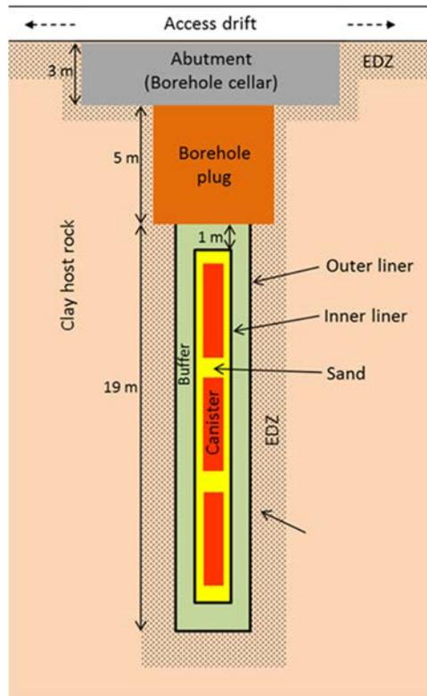
**Figure 2.2:** Illustration of the disposal concept for the northern Germany site considered in the ANSICHT test case. The borehole plug would be constructed from bentonite and the abutment would be constructed from cementitious materials. From Farrow *et al.* (2019).
