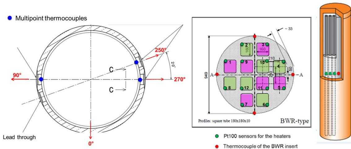
**Figure 4.5:** The locations of K-type multipoint thermocouples on the inner surface of the copper canister (left). The locations of Pt100 sensors on the canister's iron insert, and thermocouples (K-type) on the surface of the BWR insert (right). From VTT *et al.* (2019).
