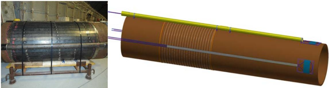
**Figure 4.13:** The steel liner used in the AHA1604 demonstrator equipped with OFS cables for monitoring strain. From Andra and EDF (2019).
