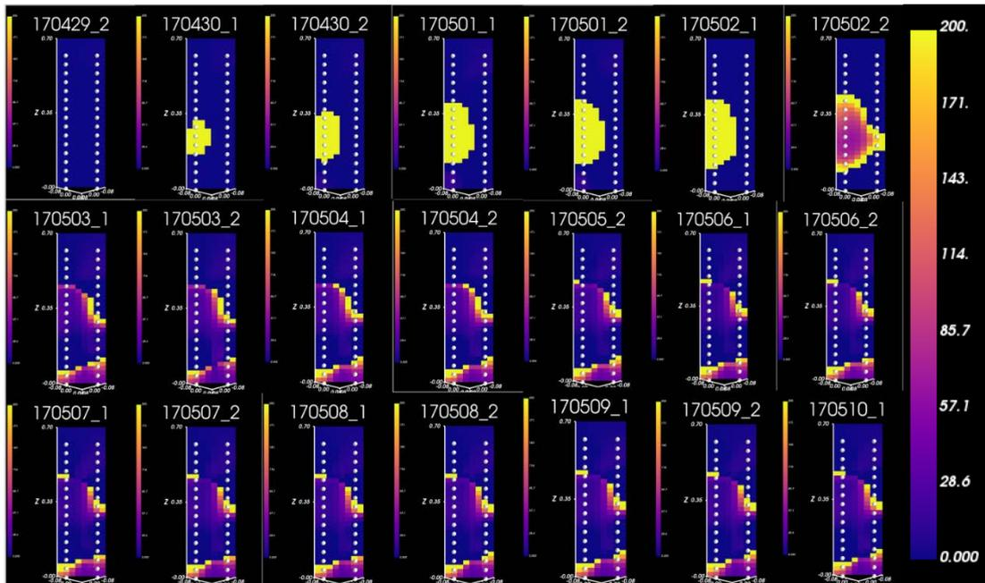
**Figure 3.9:** The PFE calculated from the 3D inverted resistance data. From ETH *et al.* (2019).
