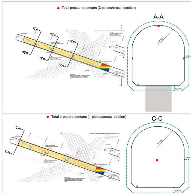
**Figure 4.9:** The locations of total pressure sensors in the backfill tunnel. From VTT *et al.* (2019).
