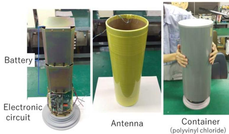
**Figure 3.2:** Conceptual design of a wireless data transmitter. From Schröder et al. (2019).
