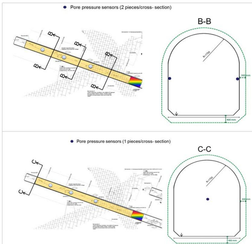
**Figure 4.10:** The location of pore pressure sensors emplaced on the backfill tunnel wall. From VTT *et al.* (2019).
