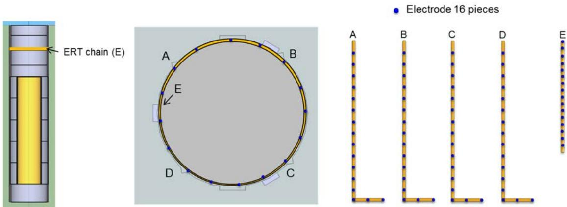
**Figure 4.8:** Locations of the ERT electrode chains in the experimental deposition hole. From VTT *et al.* (2019).
