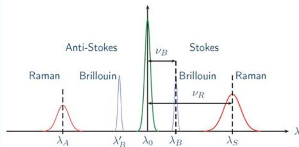
Typical spectra of waves scattered through interactions with an optical fibre.
