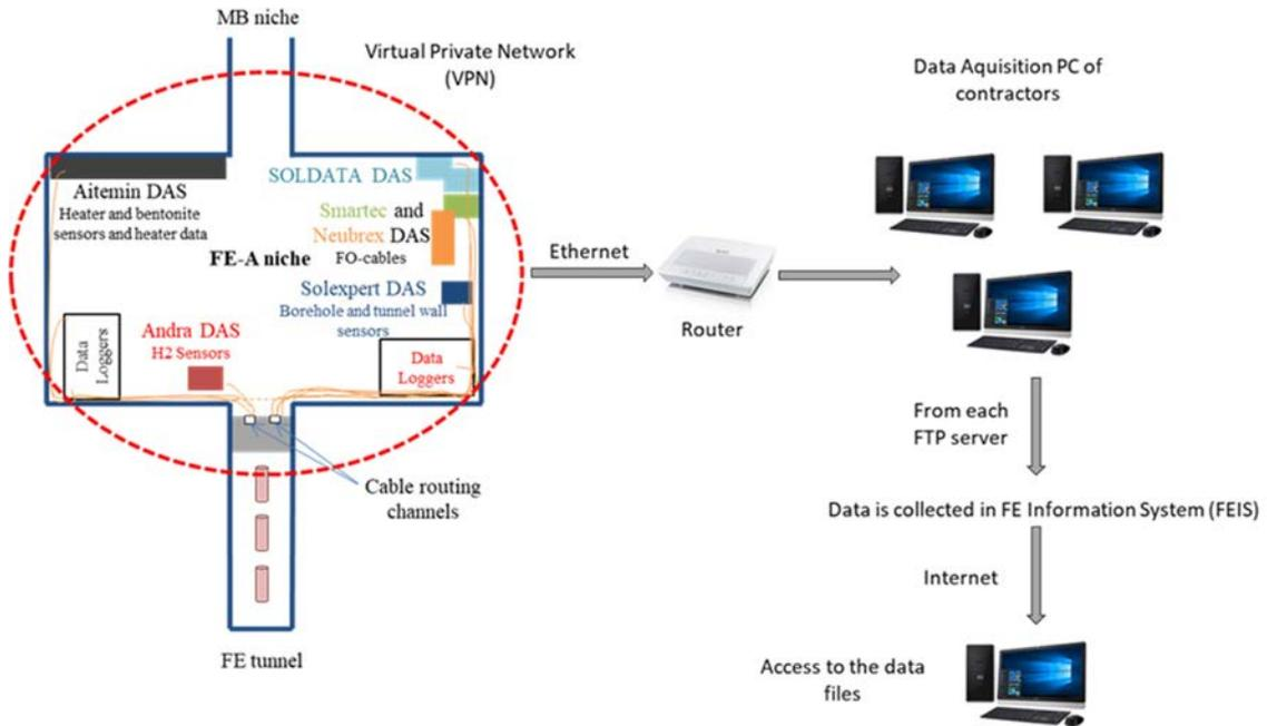
**Figure 4.24:** Illustration of the data acquisition systems installed at the FE experiment (left) and the workflow for data collection from all data acquisition systems (right). From Firat Lüthi (2018)
