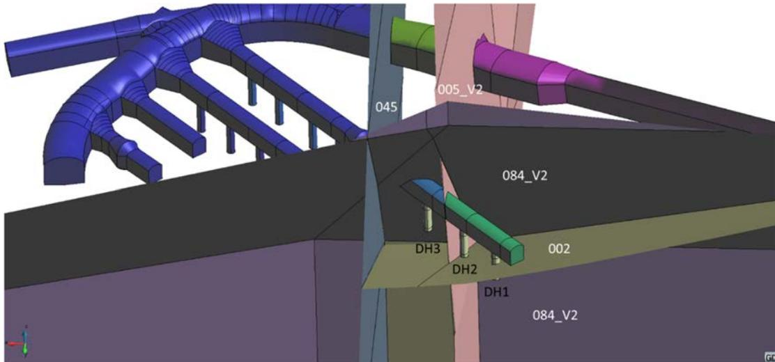
**Figure 4.2:** The geometry and location of fractures used as input to the model for its fractured case. From VTT *et al.* (2019).
