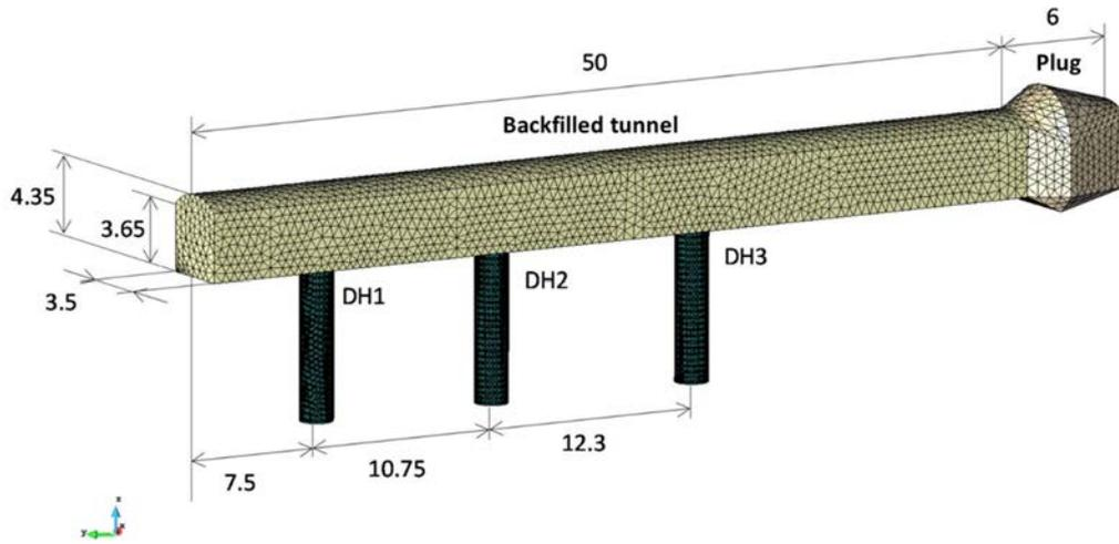
**Figure 4.1:** The experiment tunnel geometry and dimensions, as used in the thermo-hydraulic simulations for the *in situ* EBS system test. Each deposition hole (DH1 to DH3) contains a canister surrounded by a bentonite buffer. From VTT *et al.* (2019).
