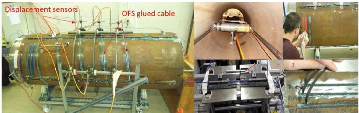
**Figure 4.14:** Photos of the sleeve equipped with OFS cables, the Sleeve equipped with (outside) classical sensors and OFS cables spiraled and (inside) hydraulic jack used to apply the radial loading (left) and the different steps of the laboratory test (1) surface preparation, (2) glue test, (3) axial strains up to break, (4) load test, and (right). The test bench is used for the calibration of the system. From Andra and EDF (2019).
