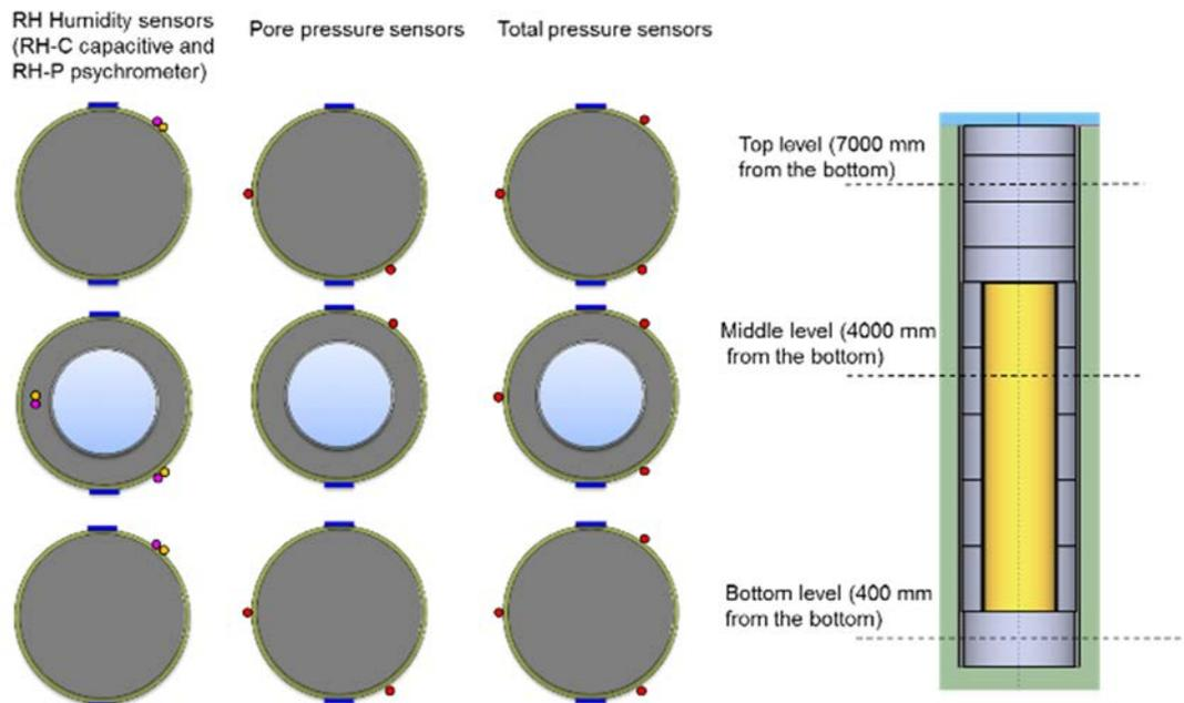
**Figure 4.6:** The locations of relative humidity, pore pressure and total pressure sensors in the deposition tunnel, on the surface of the rock. Temperature is also measured by all of these sensors. From VTT et al. (2019).
