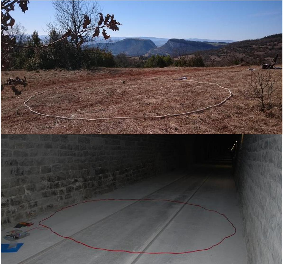
**Figure 4.19:** Data receiver on top of the surface plateau (top) and data transmitter in the Tournemire tunnel (bottom). From Dick *et al.* (2019).
