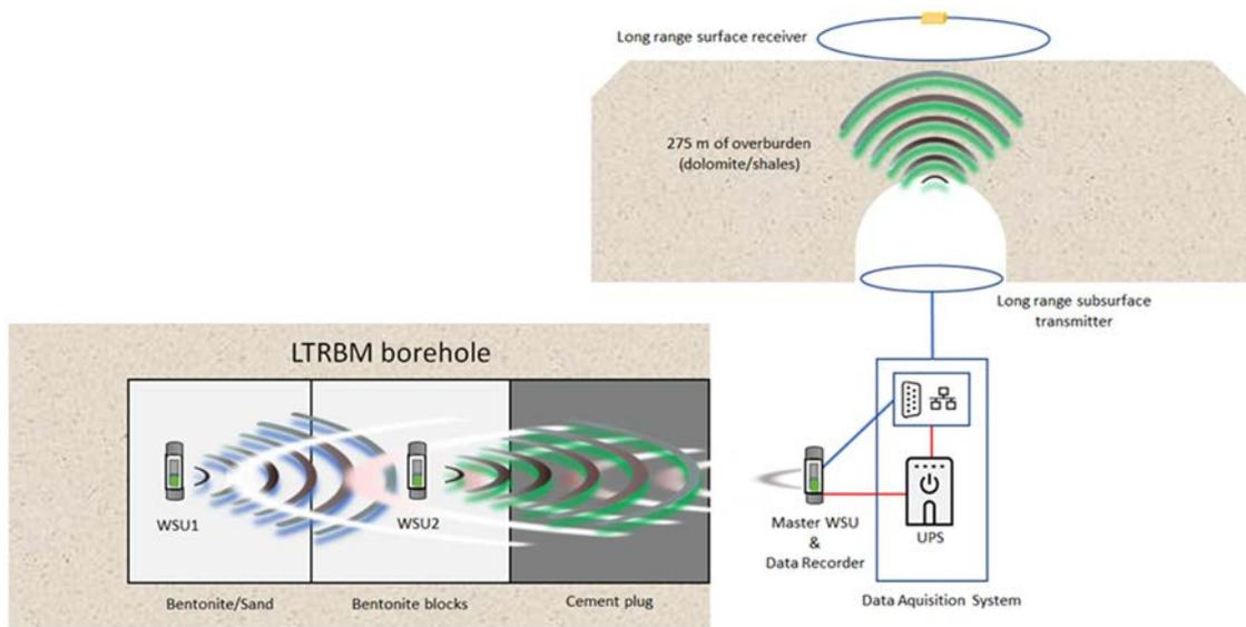
**Figure 3.4:** Overall set-up of the combined wireless data transmission chain from the LTRBM demonstrator to the surface.
