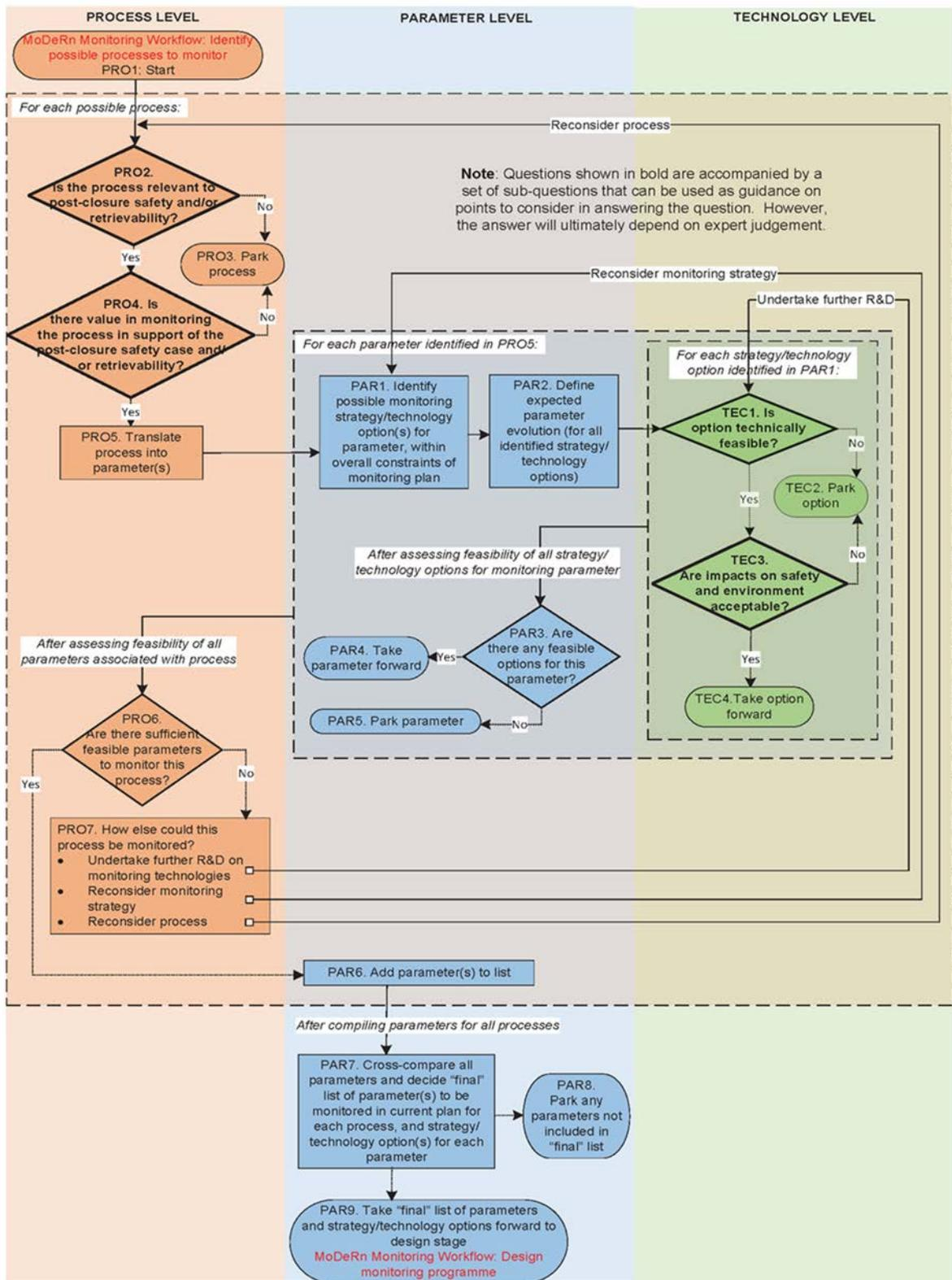
**Figure 2.7:** The Modern2020 Screening Methodology for selection of monitoring parameters.
