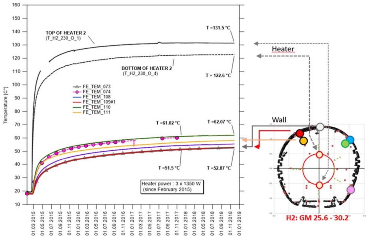
**Figure 4.23:** Evolution of the temperatures at the heaters and at the tunnel wall from 2014 to 2018. From Fisch *et al.* (2019).
