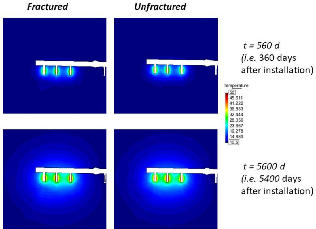
**Figure 4.3:** Temperature distribution (°C) in the rock at 360 days (top) and 5400 days (bottom) after installation, for the fractured (left) and unfractured (right) cases. From Kristensson (2015).
