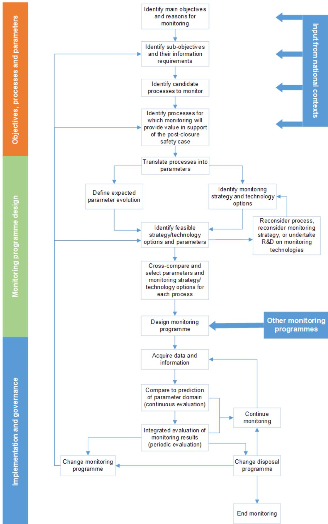
Figure 2.9: The Modern2020 Monitoring Workflow.
