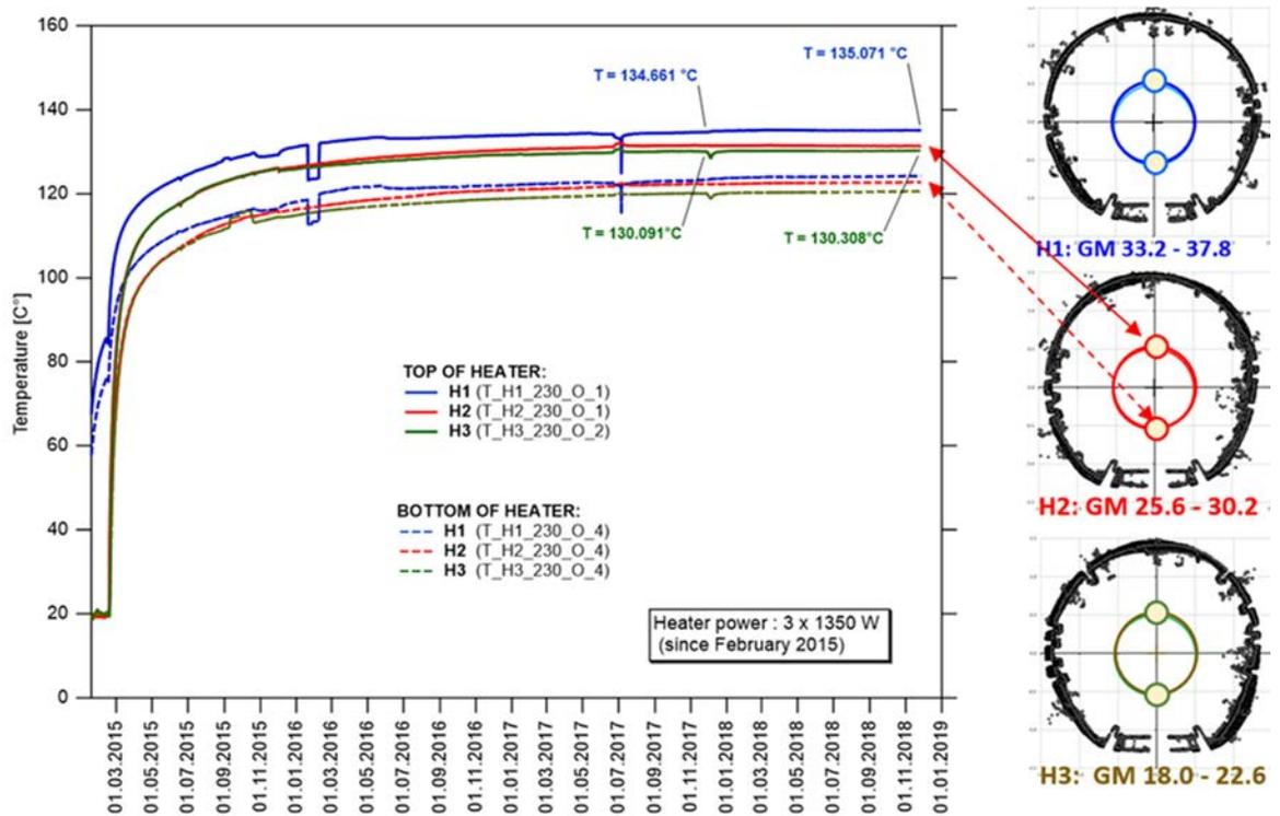
**Figure 4.22:** Evolution of the temperatures at the bottom and top side of each heater from 2014 to 2018. From Fisch *et al.* (2019).
