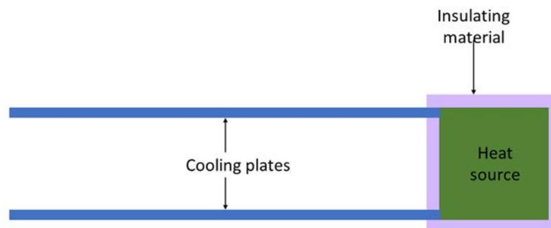
*Schematic view of an radioisotope thermoelectric generator. Cooling plates may be composed of a compound such as bismuth telluride.*
