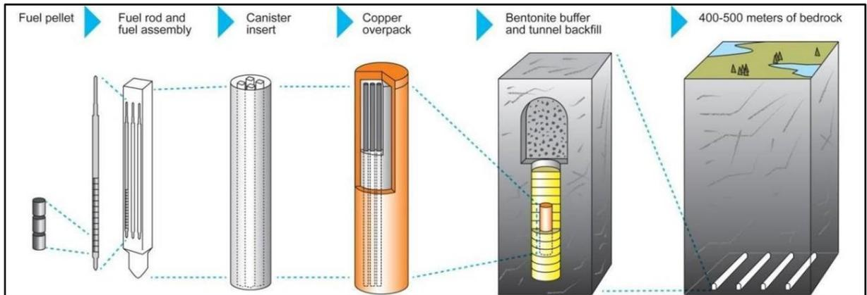
**Figure 2.5:** Illustration of the KBS-3V concept for disposal of spent fuel.
