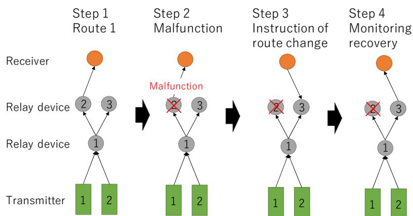
**Figure 3.3:** Conceptual diagram for a multi-hopping data relay transmission system, also illustrating the concept of route change in the case of device malfunction. From Schröder et al. (2019).
