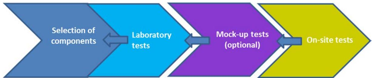
**Figure 3.12:** Global sketch for the qualification of repository monitoring components. From IRSN *et al.* (2018).
