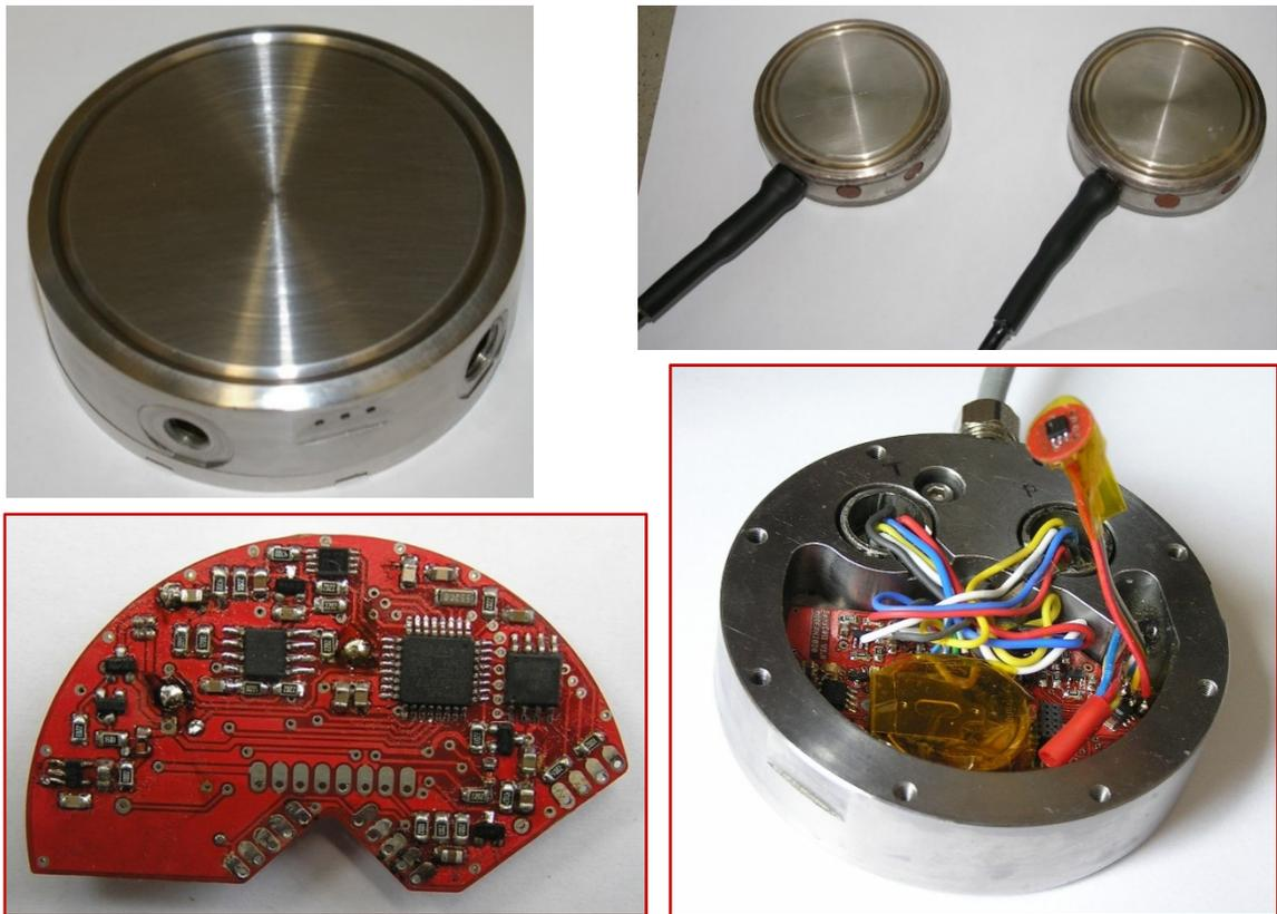
**Figure 3.7:** Photographs of the combined THM sensor. The sensor is 80 mm in diameter and 25 mm in height. From Bertrand *et al.* (2019).
