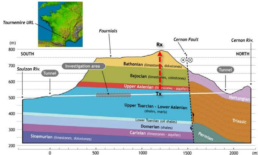
**Figure 4.16:** A cross section of the geological setting within which the Tournemire URL resides. The figure also shows the location of the long range data transmitter and receiver demonstrated within LTRBM. ‘Tx’ indicates the location of the subsurface transmitter, and ‘Rx’ the surface receiver. The transmission distance is 275 m. From Dick *et al.* (2019).
