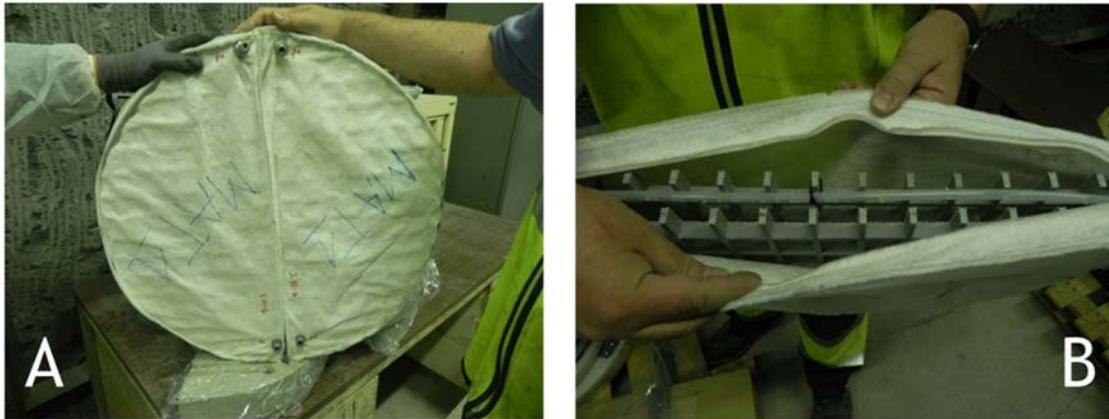
**Figure 4.18:** Photos of the hydration mats used to hydrate the bentonite buffer. (A) shows the first type of hydration mat. (B) shows the second type of hydration mat. From Dick *et al.* (2019).
