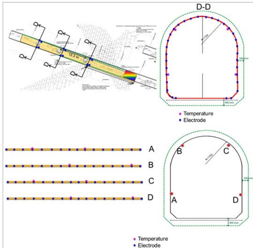
**Figure 4.11:** The locations of ERT electrode chains in the backfill tunnel, along the tunnel cross section (top) and longitudinally along the tunnel (bottom). From VTT *et al.* (2019).
