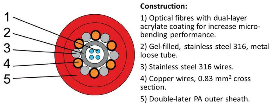
**Figure 3.6:** Schematic cross-section of the heatable fibre optic cable used to evaluate active distributed temperature sensing. From Solifos (2019).
