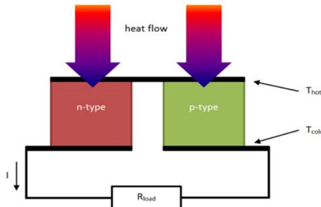
*Schematic showing the basic principles of a thermoelectric generator. Semiconductors (in this case n-type and p-type semiconductors) and the direction of heat flow are indicated.*
