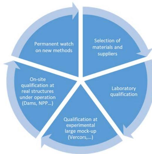
**Figure 3.10:** Selection and qualification process implemented at EDF for monitoring components. From IRSN *et al.* (2018).
