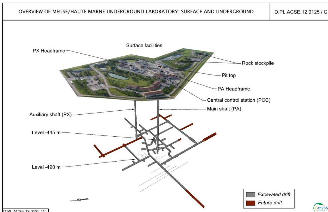
**Figure 4.12:** Overview of the Bure URL, including the surface facilities. The dashed red ellipse indicates the location of the demonstrators where HLW cells are located. From Andra and EDF (2019).
