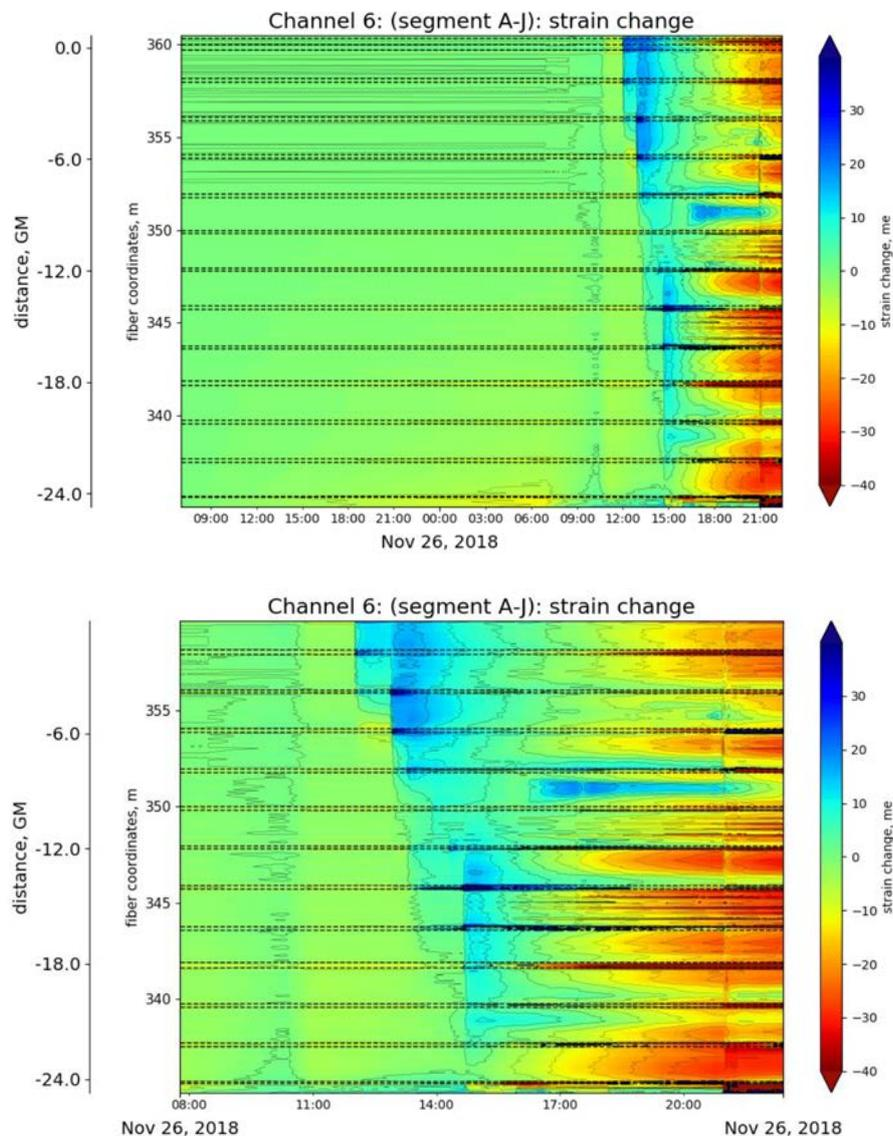
**Figure 4.15:** Strain change recorded by OF during the installation of the ALC1605 demonstrator.
