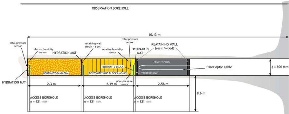
**Figure 3.1:** Layout of the WTB in the Tournemire URL. From Schröder *et al.* (2019).
