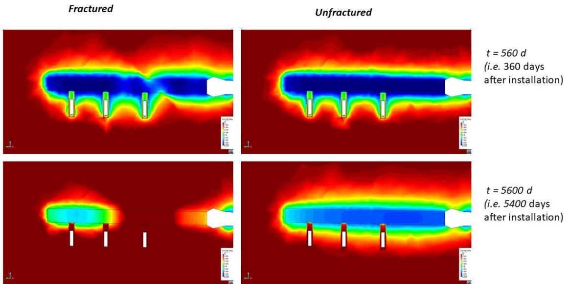
**Figure 4.4:** Vertical cross sections showing the degree of saturation in the buffer and backfill of the deposition tunnel 360 days (top) and 5400 days (bottom) after installation of the EBS, for the fractured (left) and unfractured (right) cases. Higher degrees of saturation are denoted by the red colour, and lowest degrees of saturation are denoted by the blue colour. From Kristensson (2015).
