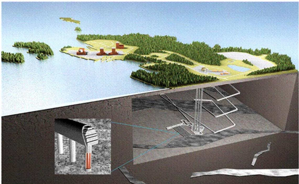
**Figure 2.6:** Illustration of the Olkiluoto repository considered in the TURVA 2012 test case. From Farrow *et al.* (2019).
