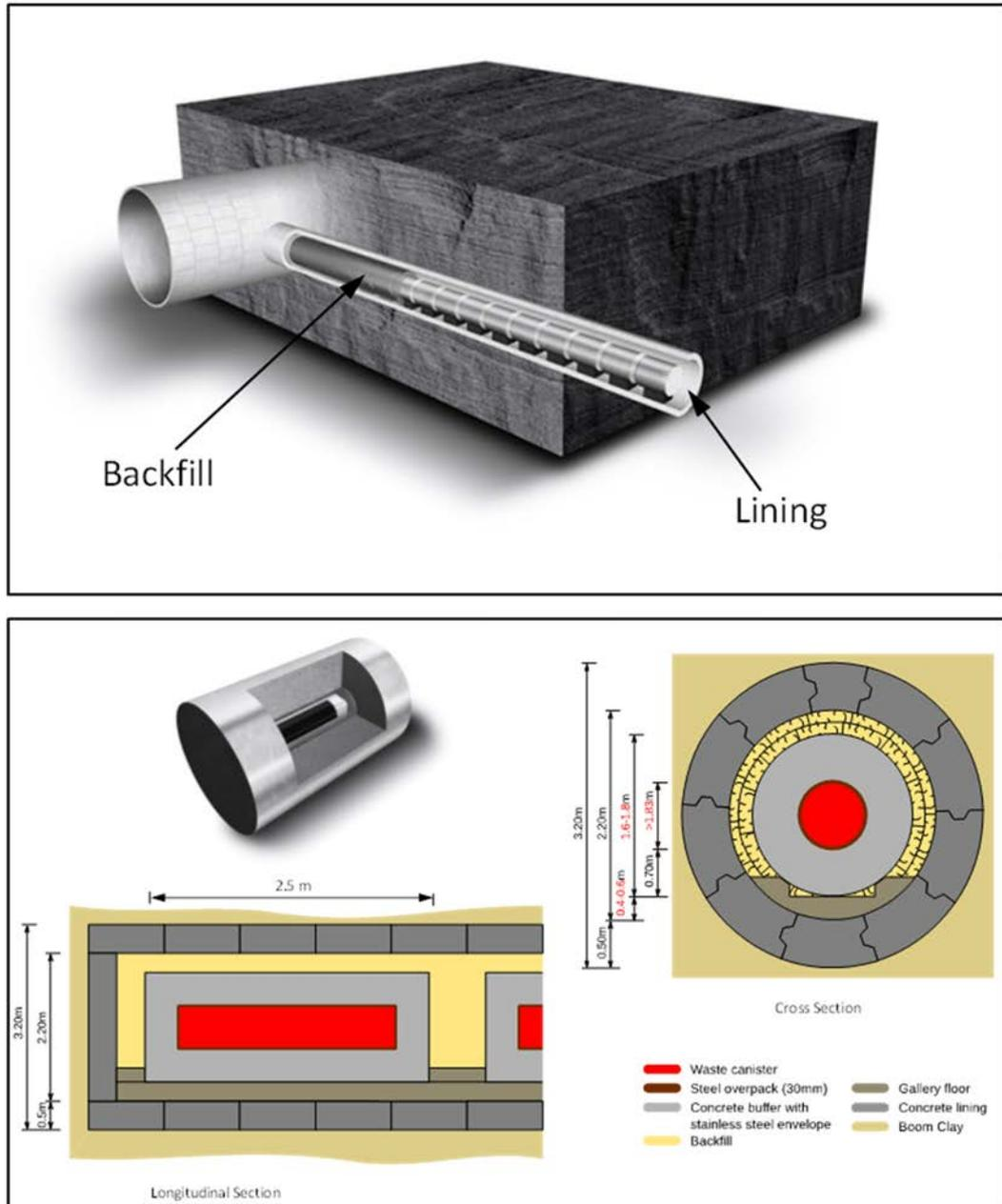
**Figure 2.4:** Illustration of the disposal concept considered in the OPERA safety case for the Boom Clay. Top figure shows the configuration of the disposal tunnels and bottom figure shows cross-sections and 3D image of the supercontainer. From Farrow *et al.* (2019).
