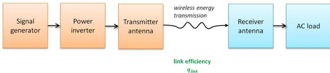
**Figure 3.5:** The wireless energy transmission set-up used in the pilot scheme involving a high-electrical-conductivity medium. From Strömmer et al. (2019).
