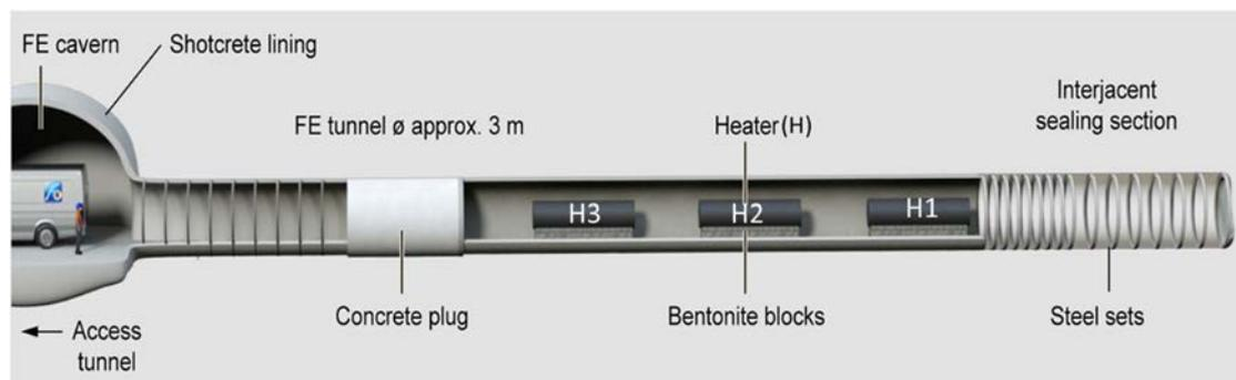
**Figure 4.20:** Experimental layout of the FE Experiment. The main parts of the FE cavern and FE tunnel are shown here without backfill. From Müller *et al.* (2017).
