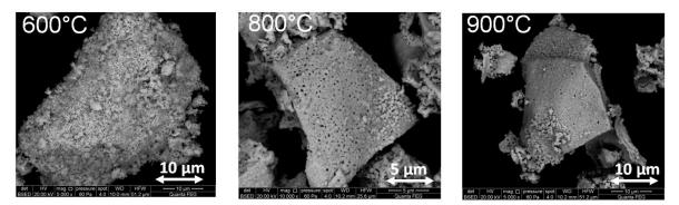
Fig.3.1.2. TEM images of U3O8 after oxidative sintering at different temperatures
