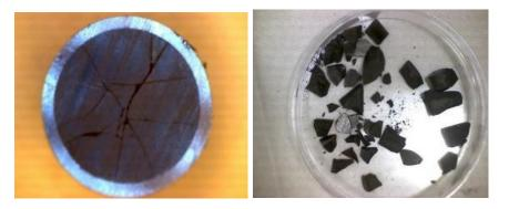
Figure 2.1.1 (a) cut pellet with zircaloy cladding (b) fragments for leaching experiments
