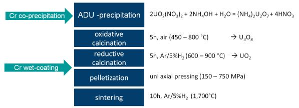
Figure 3.1.1. Principal scheme of wet chemical synthetic rout for pure and Cr-doped UO<sub>2</sub>
