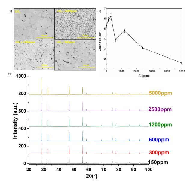
Figure 4.1.1 Analysis of Al-doped  $UO_2$  prepared via wet synthesis route I, showing: (a) images of the  $UO_2$  and Al-doped  $UO_2$  microstructure as obtained by SEM; (b) average grain size as a function of Al dopant concentration, as analysed by image processing using Fiji software (minimum number of grains analysed was 500); and (c) X-ray diffraction patterns for Al-doped  $UO_2$ . Rietveld refinement of these data showed no influence of Al-doping on the lattice parameter of  $UO_2$ .
