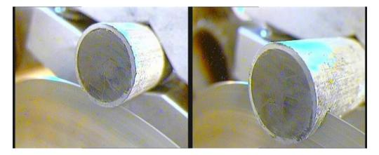
Figure 2.2.1: cutting of MOx pellets (a) MOx-H (b) MOx-L
