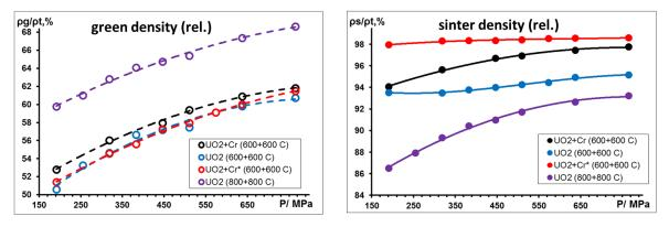
Figure 3.1.3. Density of  $UO_2$  pellets as a function of calcination temperature and pressure. The temperatures of stages 2 and 3 (Fig.3) are given in brackets for each experiment set.
