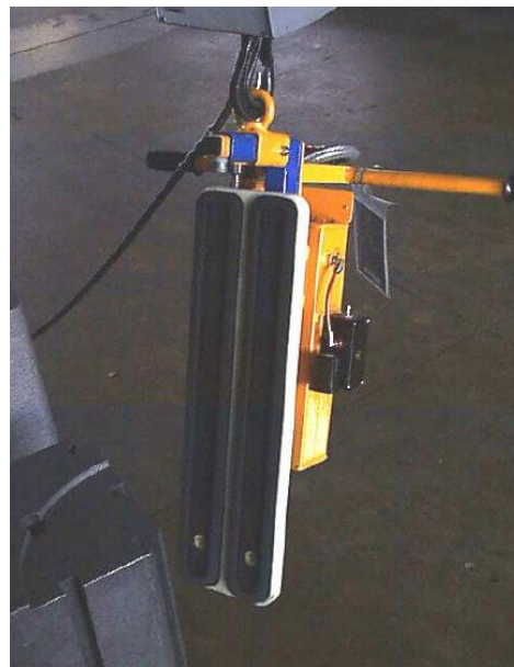
Figure 8: Vacuum system for graphite bricks handling device
