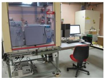
Figure 8: Gas chromatography-coupled with mass spectrometry.
