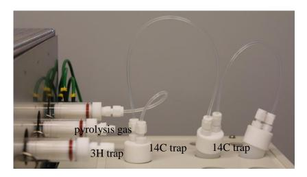
Figure 5: System to trap the pyrolysis gases.
