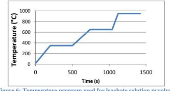
Figure 6: Temperature program used for leachate solution pyrolysis.
