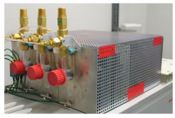
Figure 3: Tri-tube pyrolysis furnace.
