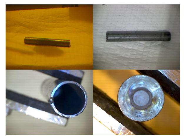
Figure 8 Irradiated Zry-4 plenum specimen used for the dissolution experiments
