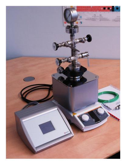
Figure 7 Autoclave with heating mantle and hot plate for assuring a constant temperature during the leach tests
