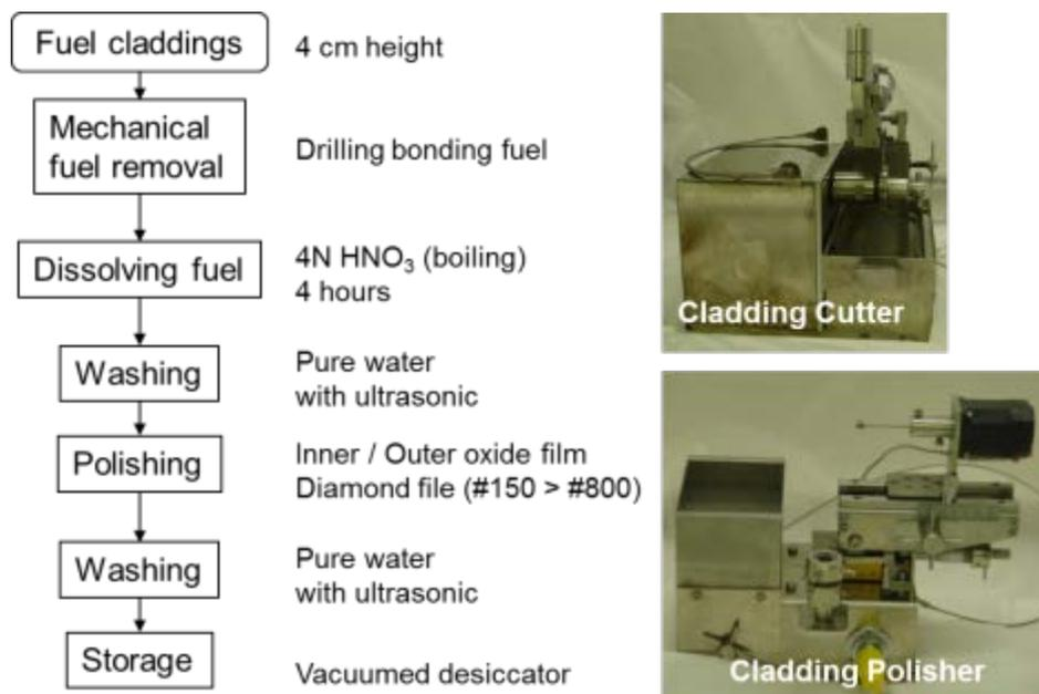
**Figure 11 : Pretreatment for specimens.**
