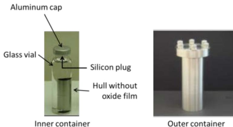
**Figure 13 : Pictures of the test containers.**
