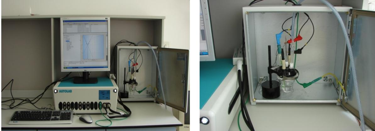
**Figure 11: Electrochemical set-up.**
