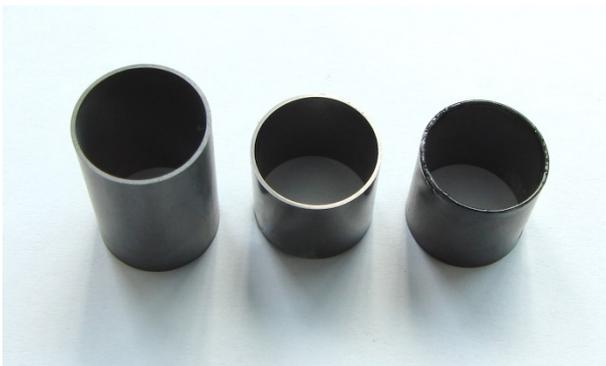
**Figure 12. Oxidised Zy-4 tube uncut (left), oxidised Zy-4 tube cut at the end (middle) and oxidised Zy-4 tube cut and painted (right).**
