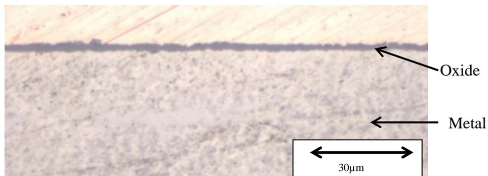
**Figure 9: Oxide layer thickness measured by optical microscopy (magnification x1000).**
