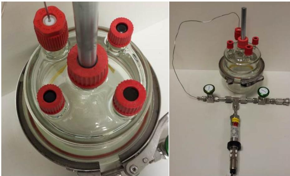
**Figure 6: Glass cell for LPR test setup.**
