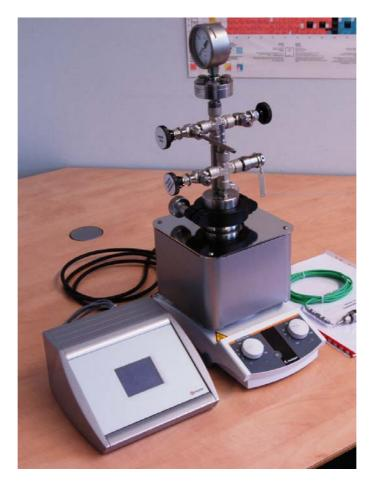
Figure 6.1: Autoclave with heating mantle and hot plate for assuring a constant temperature during the leach tests
