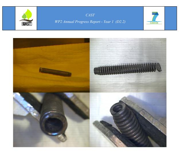
Figure 7.1: Irradiated stainless steel plenum spring used for the dissolution experiments
