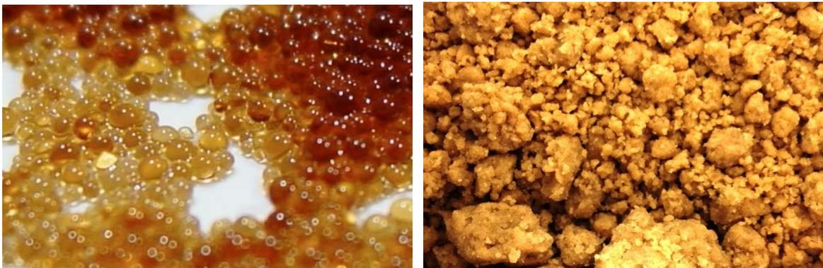
**Figure 5. Comparison among IERs in bead form (left) and powder form (right, flocculated).**
