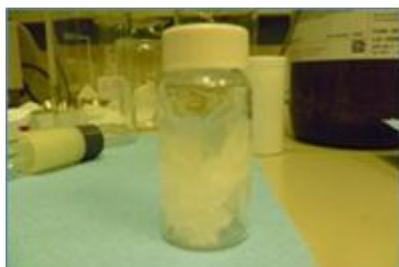
**Figure 19. Formation of gel colloidal during the adsorption of CO<sub>2</sub> in amine without the addition of methanol.**
