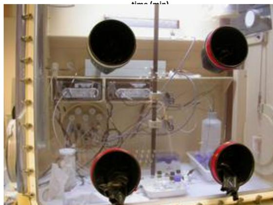
**Figure 31. Example of a chromatogram obtained in cementitious conditions (a), and photograph of the ion chromatography set-up in glove box (CEA).**
