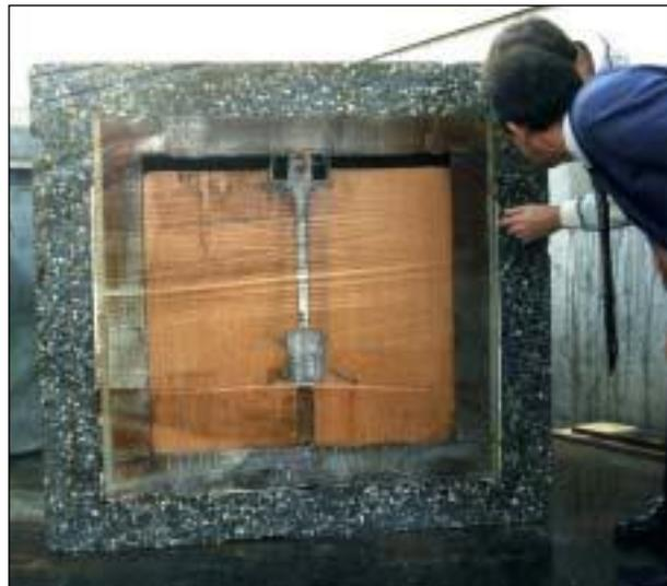
**Figure 2: Cross section of a “Mercure” C1PG package (SOCODEI).**
