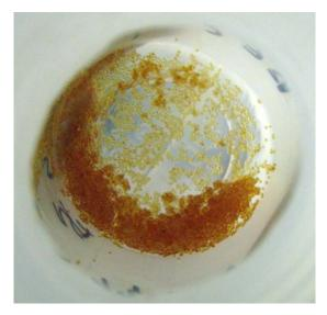
Figure 4. SIER from ÚJV Group research reactor operation
