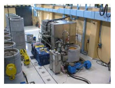
Figure 9. Mobile unit used for SIERs conditioning on-site.
