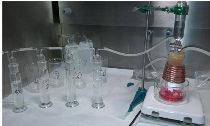
**Figure 18. The modified experimental set-up for  $^{14}\text{C}$  acid stripping in INR**
