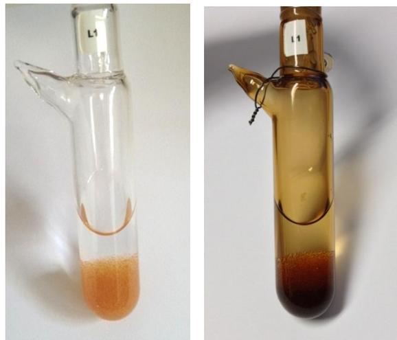
**Figure 15. Sample vials filled with anion exchange resins and water, before (left) and after irradiation campaign (right) (FZK).**
