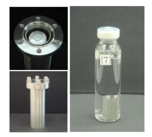
Figure 16 External view of outer vessel (left) and cladding immersed in glass vessel (right) for long-term static leaching test.
