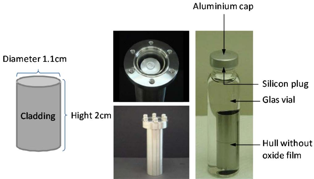
Figure 19 Vessels of corrosion test for irradiated Zircaloy-2.
