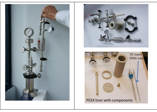
Figure 3.5: Berghof autoclave (left) with its gas sampling vessel, and a view of its internal components (right)
