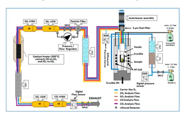
Figure 3.2 ICARUS device operating principle
