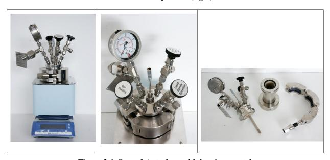
Figure 3.6: Second Autoclave with heating mantel
