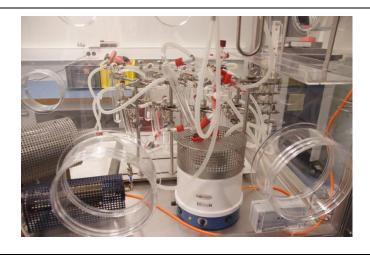
Figure 3.8: Views of the Completed Glove box for <sup>14</sup>C sample preparation.
