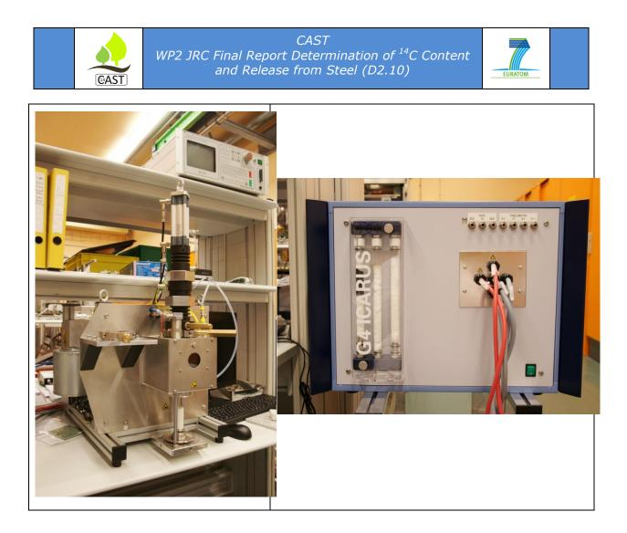
Figure 3.3 Icarus device separated into 2 components
