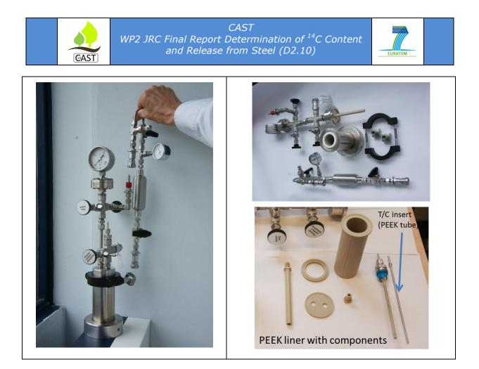
Figure 3.5: Berghof autoclave (left) with its gas sampling vessel, and a view of its internal components (right)
