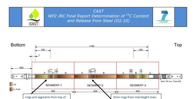
Figure 2.1 Cutting plans for steel sample rings from NIMPHE 2 pins
