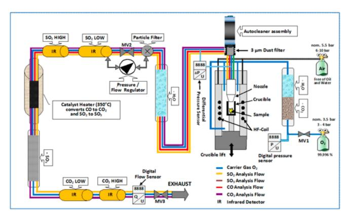
Figure 3.2 ICARUS device operating principle
