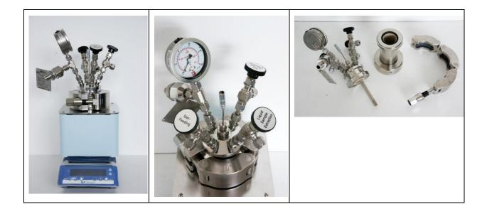
**Figure 3.6: Second Autoclave**
