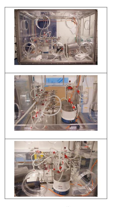
Figure 3.8: Completed Glove box for <sup>14</sup>C sample preparation.
