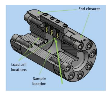
Figure 2-3. diagram showing a cross section of the vessel showing the location of the samples and load cells.
