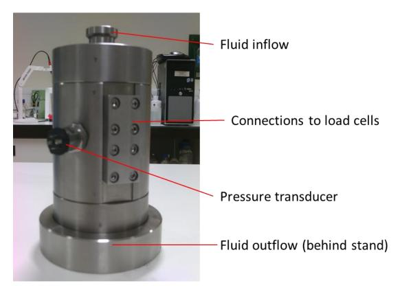
*Figure 2-1. Photograph of one of the titanium vessels constructed for this project.*
