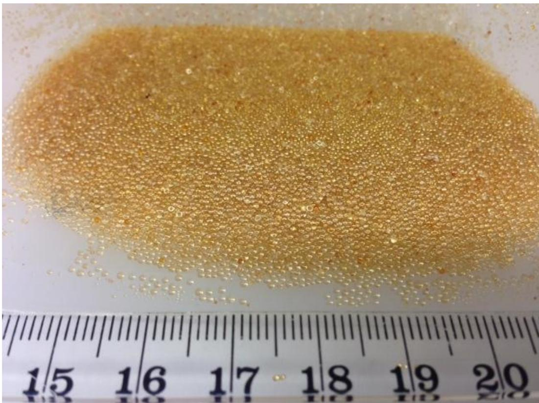
Figure 4. IXR used in CFB gasification test trials (scale is in cm).
