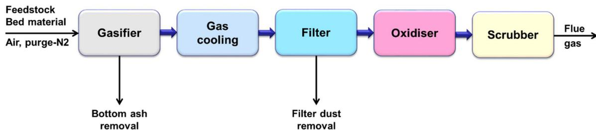
Figure 1. Principle of the gasification based thermal treatment facility (patented by VTT).
