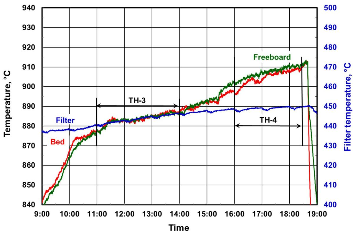
Figure 6. Gasification and filtering temperatures during 10.10.2018.
