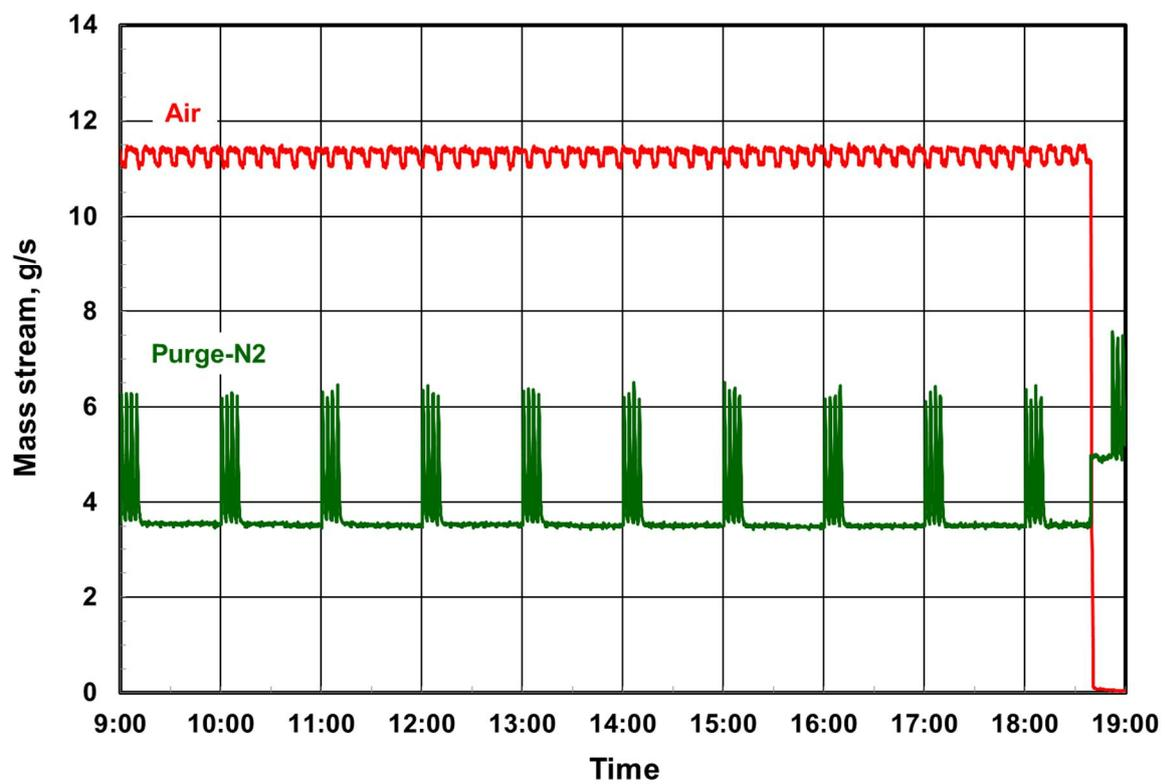
Figure 8. Air and purge-N<sub>2</sub> feed rates during 10.10.2018.
