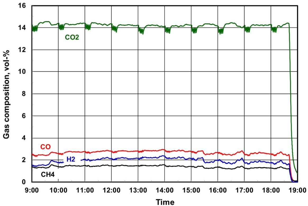
Figure 7. Main gas composition during 10.10.2018 (the main gas component is nitrogen, which is not shown in the figure).
