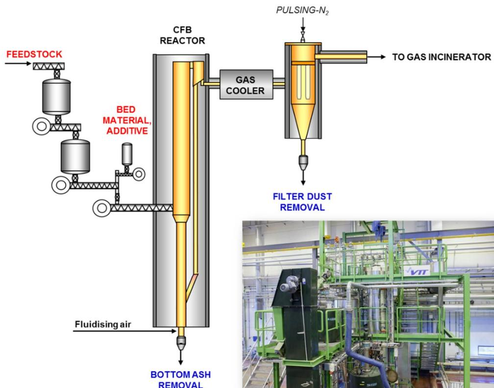
Figure 3. Pilot-scale Circulating Fluidised-Bed (CFB) gasification test rig.
