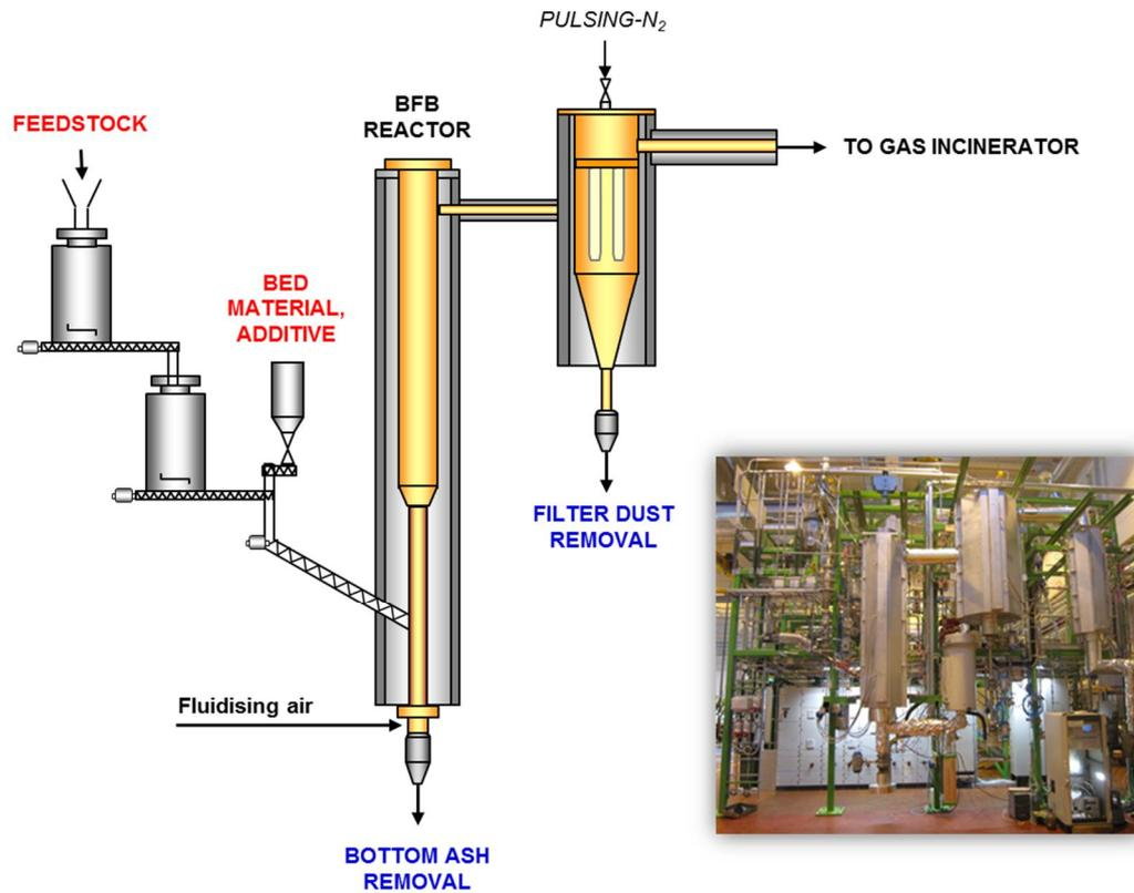
Figure 2. Bench-scale Bubbling Fluidised-Bed gasification test rig (BFB100).
