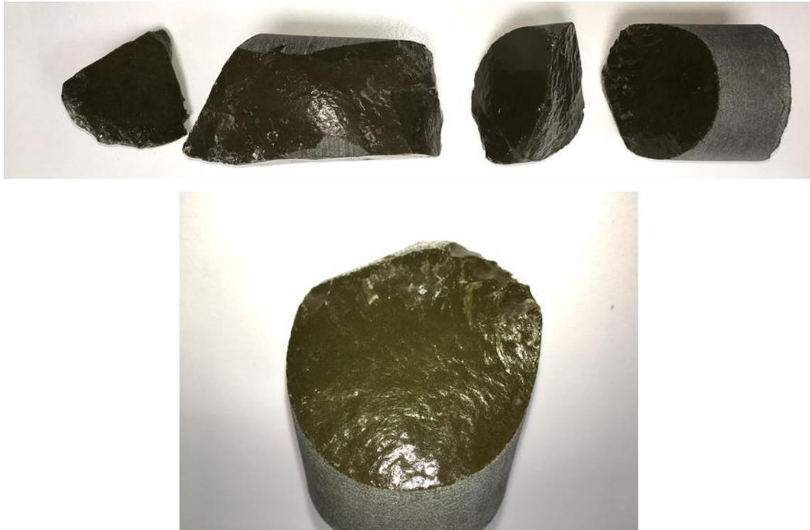
*Figure 15: Coring of the wastefrom from the In-Can Melter trial.*
