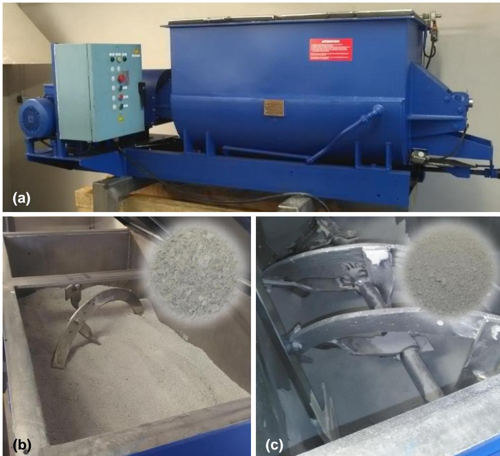
Figure 7: (a) Morton Mixers ribbon blender. Ash in the blender (b) before and (c) after homogenization.
