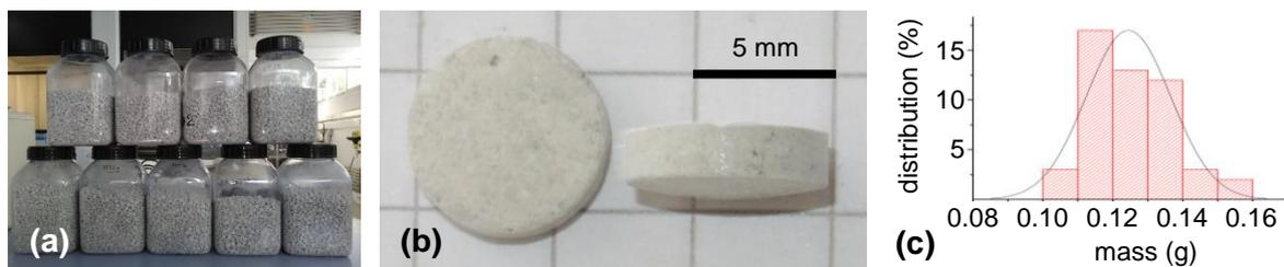
Figure 8: (a) Total production of 60,000 pellets, (b) detail view of an ash pellet and (c) mass distribution of a sample of 50 pellets.
