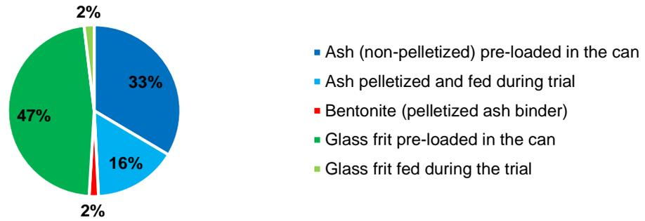
Figure 13: Distribution of the feeds in the In-Can trial
