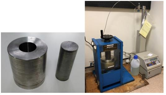
Figure 3 Steel former and plunger (left) were inserted into the hydraulic press (right) to prepare the sample to a known dry density.
