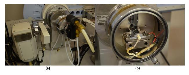
Figure 6 Configuration of PANalytical X'Pert Pro diffraction system for analysis of oriented mount samples using an Anton Paar THC (controlled temperature and humidity) chamber; (a) analytical configuration, (b) close-up of the interior of chamber showing sample position with humid air supply tubing and chamber cover removed.
