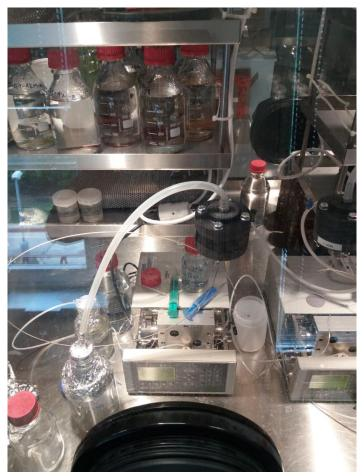
Figure 2-7. Saturation of bentonite sample in the anaerobic glove box
