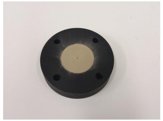
Figure 2-4. Cell body with compressed BaM bentonite, diameter 40 mm
