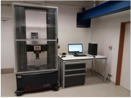
Figure 2-3. Laboratory with pressure source MTS Exceed E45
