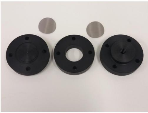
Figure 2-5. Dismantled complete cell consist of top lid, cell body, bottom lid and two stainless steel sieves
