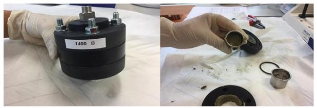
Figure 2-8. Cell filled with bentonite of density 1400 kg/m<sup>3</sup> (left) and using the ring cutter for the bentonite sampling (right)
