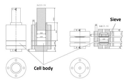
Figure 2-1. The scheme of arrangement for bentonite pressing into the cell (left) and complete cell design (right)
