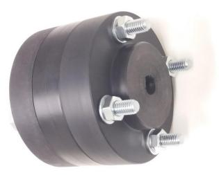
Figure 2-6. Assembled complete cell with bentonite prepared for saturation
