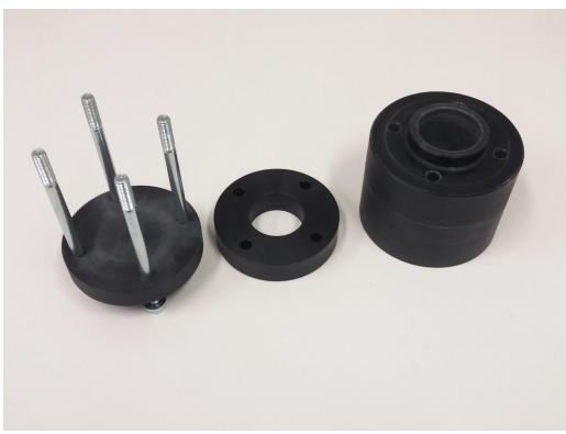
Figure 2-2. Dismantled assembly for bentonite pressing (cell body in the middle)
