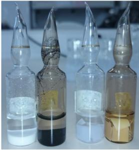
Figure 1: The effect of radiation on the appearance of PVC materials. Imaged are flame-sealed vials containing saturated Ca(OH)2 and (from left to right) non-irradiated PVC powder; irradiated PVC powder; non-irradiated PVC sheet; irradiated PVC sheet. Note the change in colour of the PVC powder from white to black, and of the PVC sheet from clear translucent to light brown opaque.
