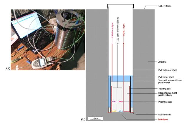
Figure 1 – View of the heating coil device connected to the temperature monitoring system (a) and outline of the CEMTEX in situ device (b).
