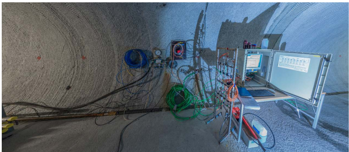
Hydraulic double packer tests in the 197 m deep ADUS Borehole
