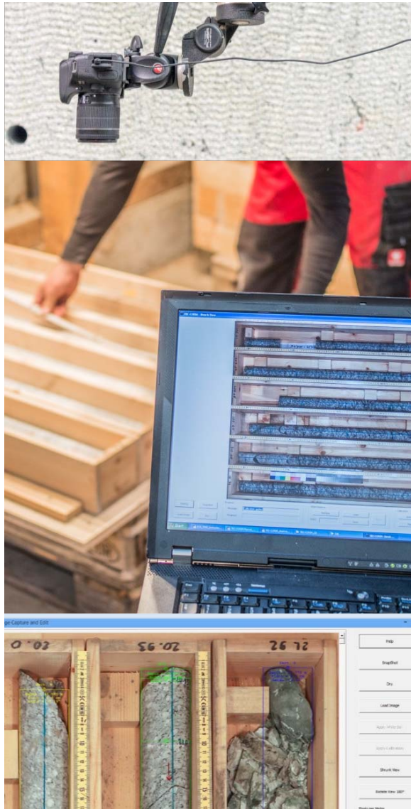
Analysis of drill cores, preparing core pictures for transfer to WellCAD
