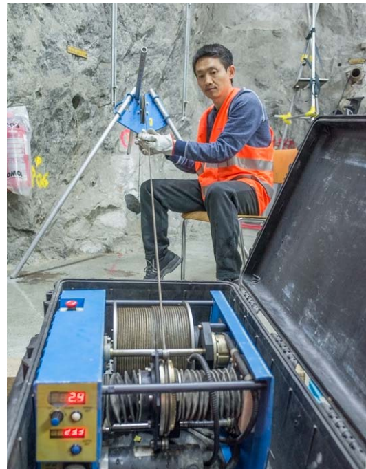
Hydraulic testing using double packer system and borehole geophysical logging.
