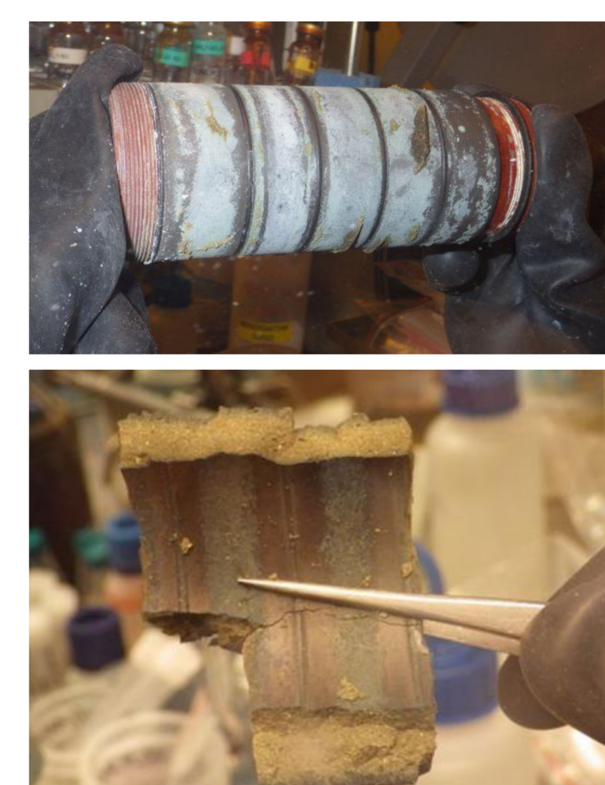
Fig. 3 Dismantled module (up) and the metal sample after 1 year exposure (in anaerobic box)
