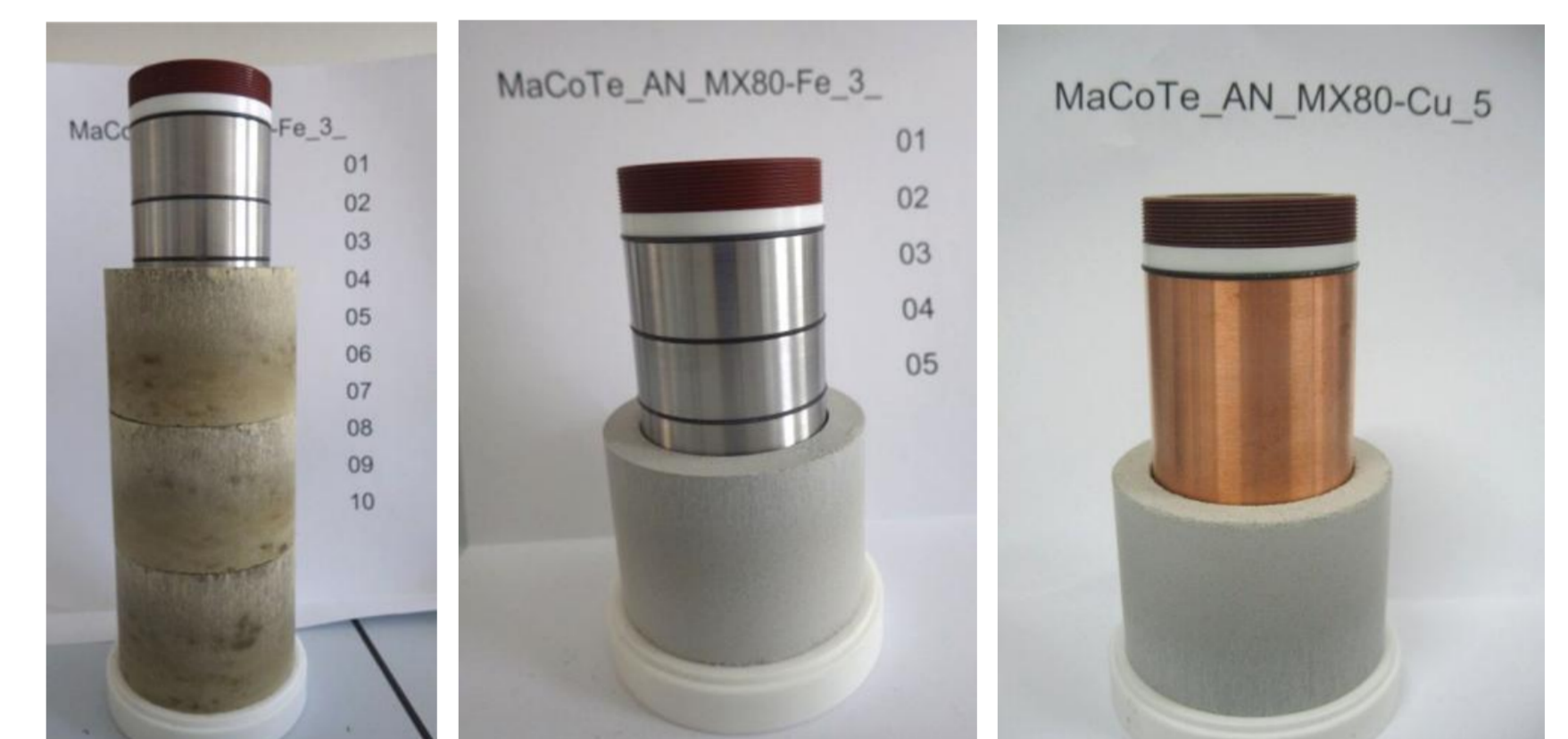
Fig. 1 Modules used in heated material corrosion test (from the left): Czech bentonite + carbon steel, MX80 + carbon steel, MX80 + Cu coating.
