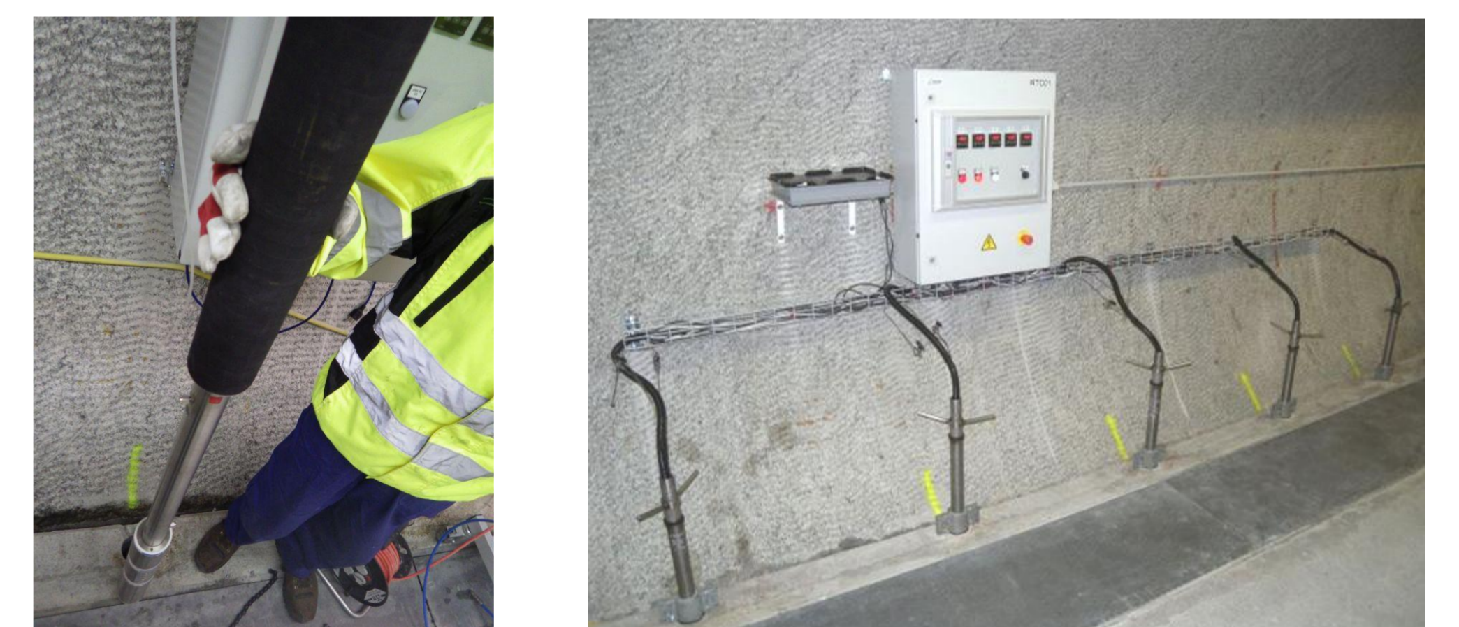
Fig. 2 Corrosion modules (left) instrumented into the boreholes at the start of the experiment in GTS (right)
