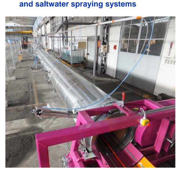
Overall view of test bench with heating
