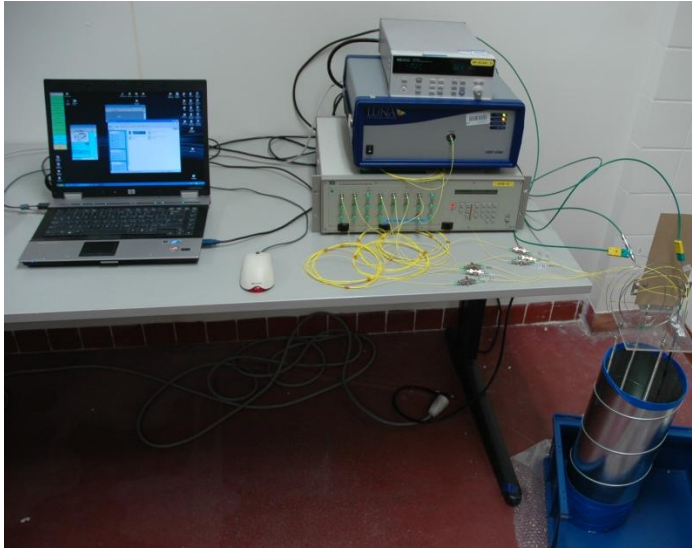
Figure 5-3-10: Set-up to test optical fibre compatibility with cast concrete
