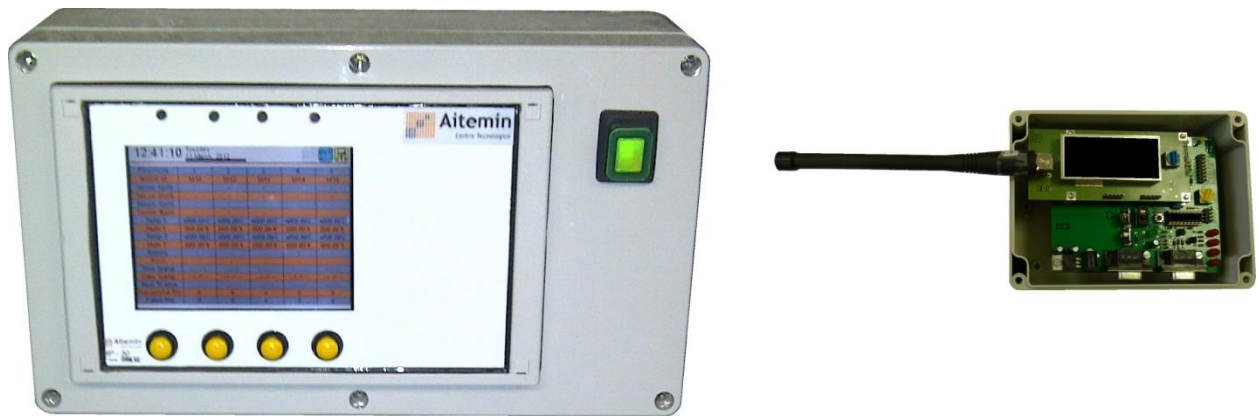
Figure 5-2-3: Wireless master controller and HFW node prototype
