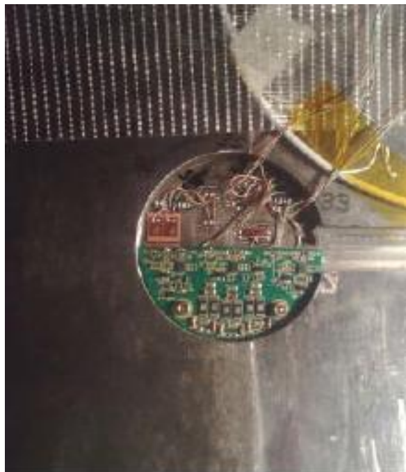
Figure 5-5-3: Instrumented sheet welded to the bottom of an internal spot facing and to which stress gauges have been attached (with 3 directions of measurement) together with their electronic components
