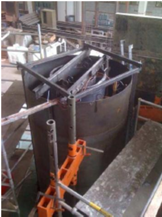
Figure 5-3-8: Setup of the half-scale tests: view of the assembled mould before casting of the buffer (left); schematic view showing the buffer and overpack/heater (right)
