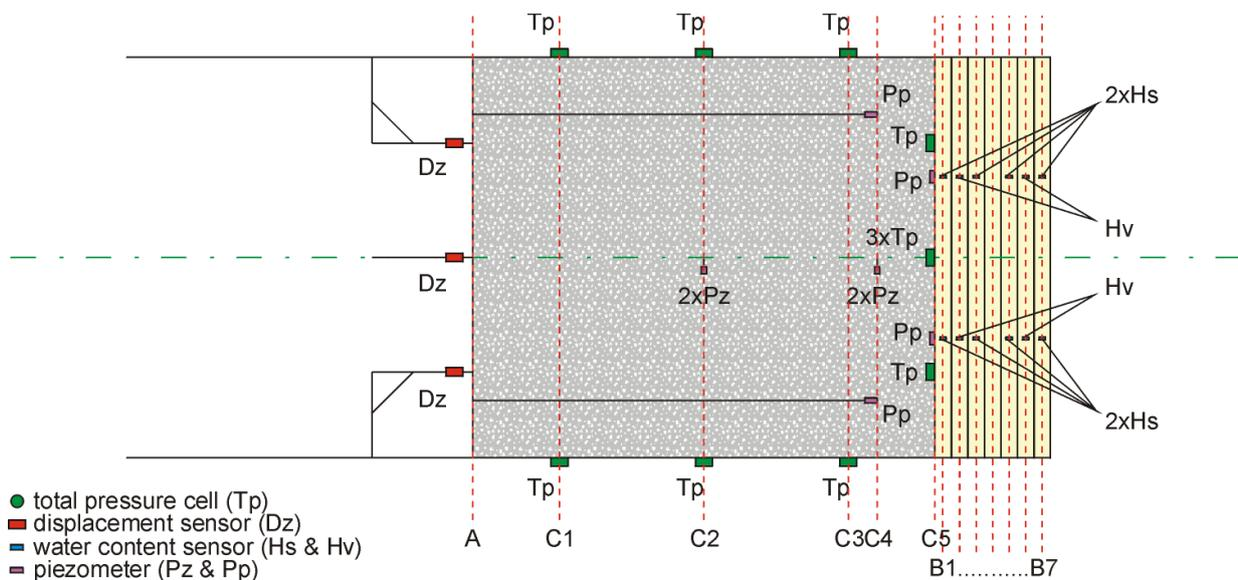
**Figure 6:** Layout of instrumentation (wired transmitted sensors only)
