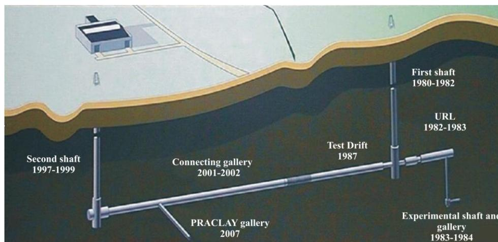
**Figure 8:** Schematic diagram of the layout and historical development of the PRACLAY Gallery in HADES URL.
