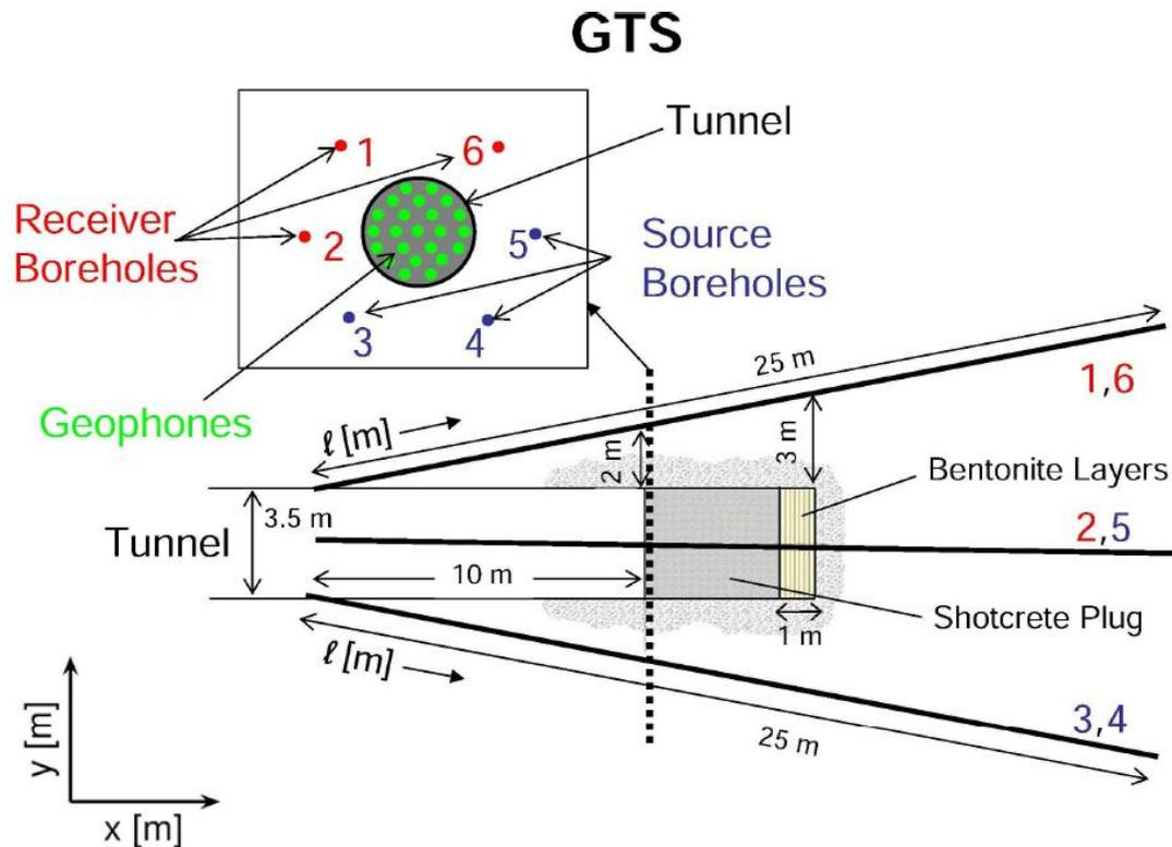
**Figure 2:** The experimental setup at the Grimsel Test Site (GTS).
