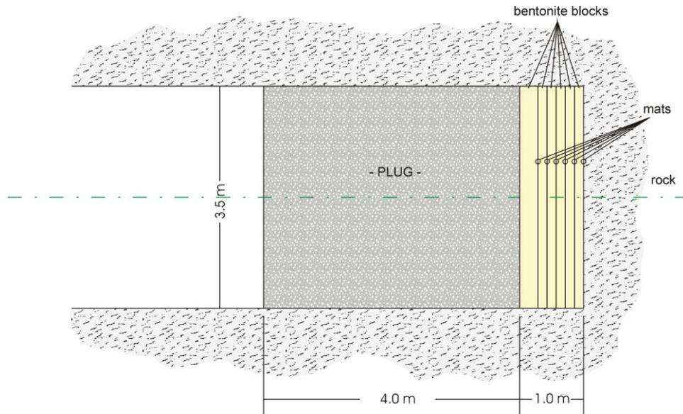
**Figure 5:** General layout of the full-scale test.
