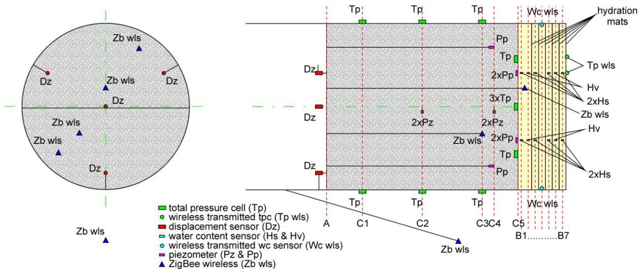
**Figure 7:** Layout of wireless instrumentation to be installed. N.B.: This preliminary layout could be changed upon the results obtained from WP2.
