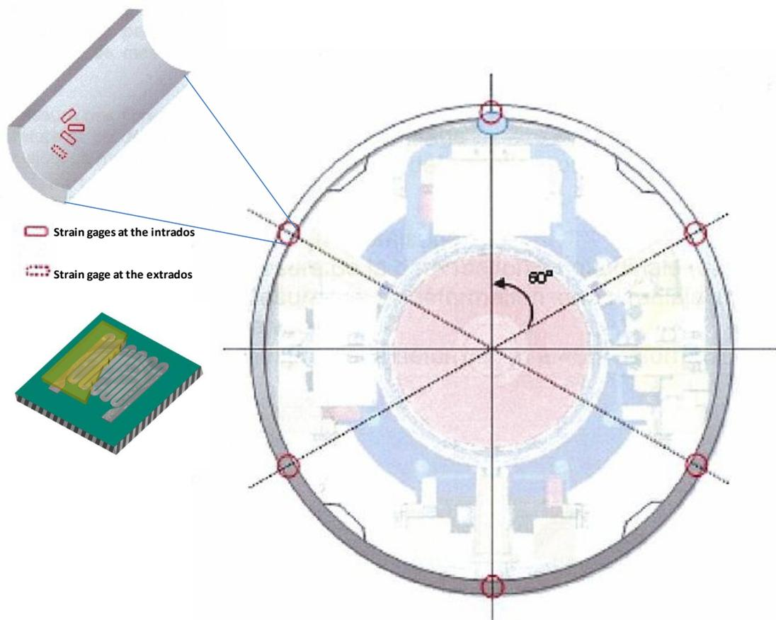
**Figure 11:** Displacement monitoring sensors on cell liner section
