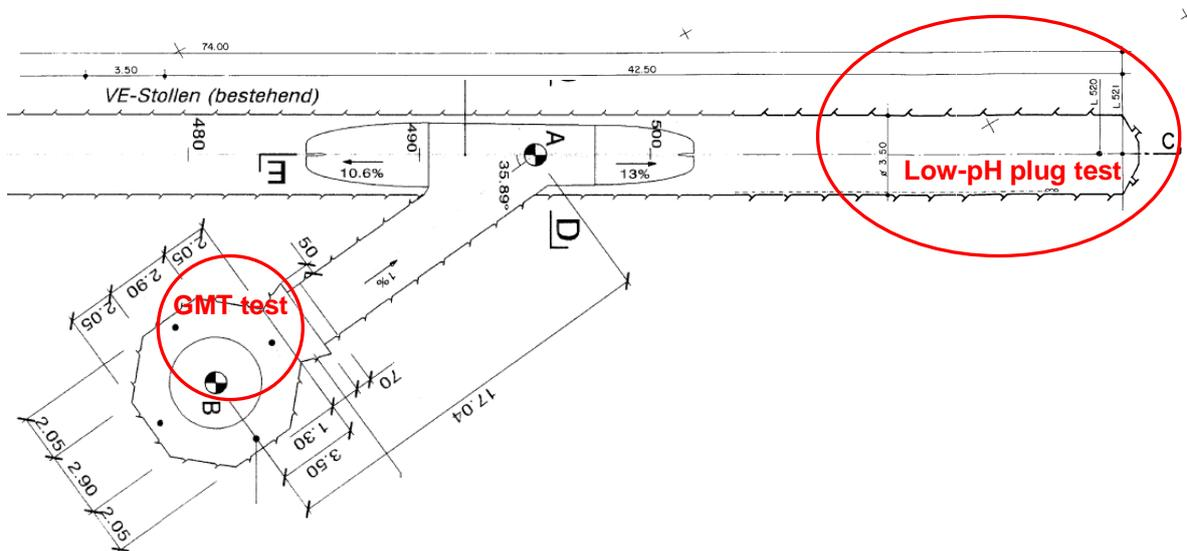
**Figure 4:** Location of the full-scale test at VE tunnel.
