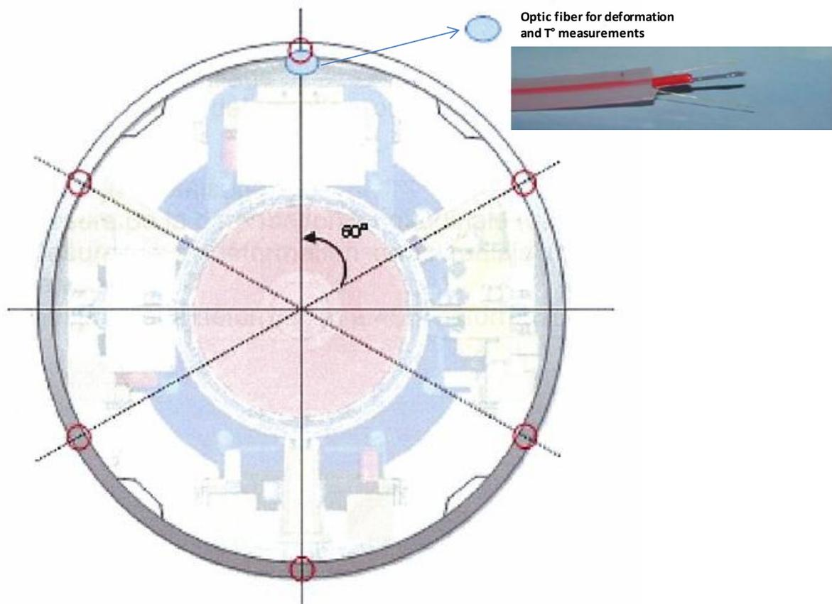
**Figure 12:** Illustration for fibre optic sensor position inside cell liner
