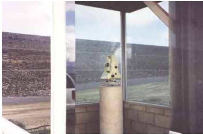
Figure 127- Robotic total station for automatic dam displacement monitoring in its shelter. (Image credit: Department of Geodesy and Geomatics Engineering, Univ. of New Brunswick)
