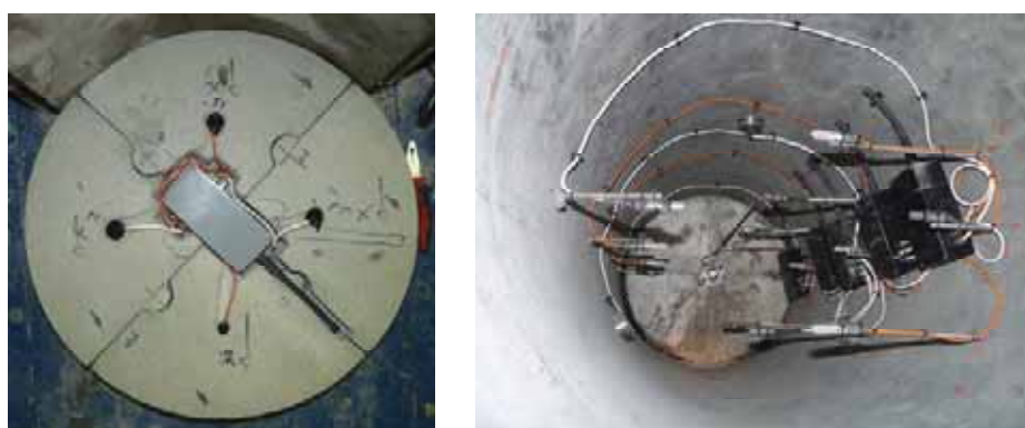
Figure 93: Appearance of node embedded in bentonite block made of four sectors (left) and nodes and instrumentation secured to the rock prior to fill up with bentonite pellets and powder (right).
