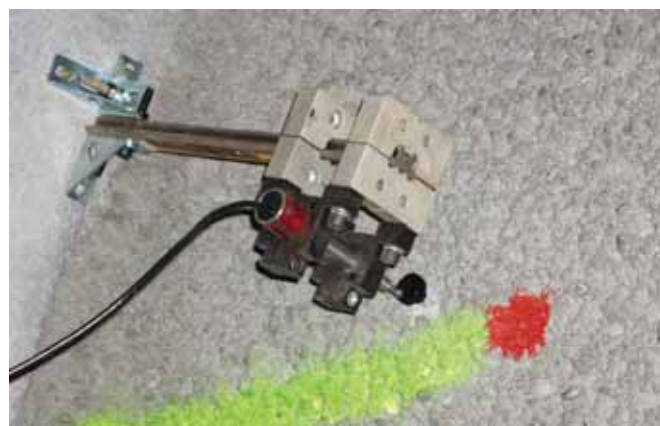
Figure 33: LVDT for measuring concrete seal displacement in ESDRED experiment
