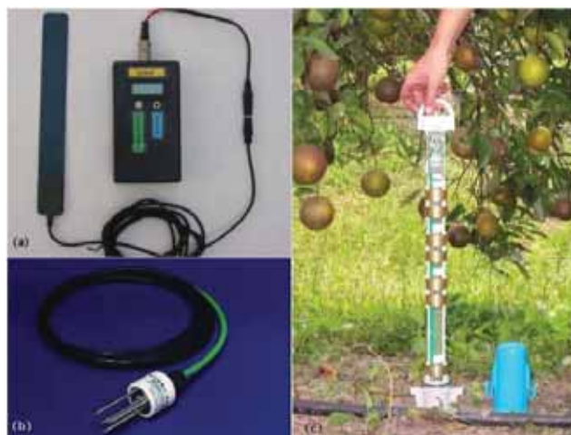
Figure 14: Frequency domain (FD) probes: a) capacitance (plates embedded in a silicon board); b) capacitance (rods); and c) FDR (rings).
