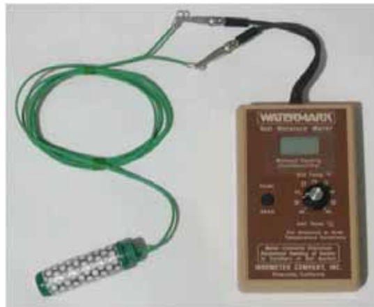
Figure 24: Granular matrix sensor (GMS) resistance block and reader
