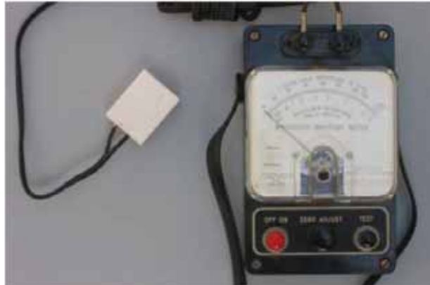
Figure 23: Gypsum (Bouyoucos) resistance block and reader
