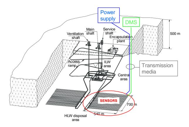
Figure 1: Layout of a generic monitoring system<sup>2</sup>
