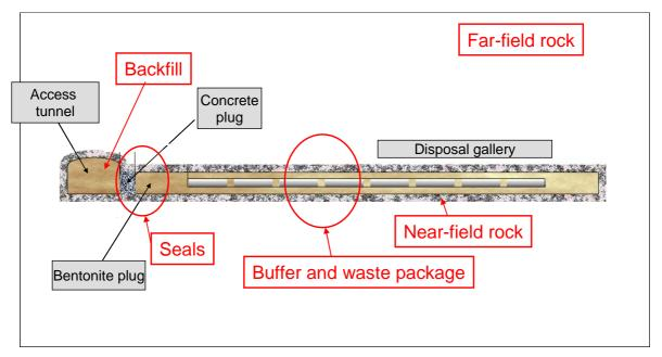
Figure 2: Schematic of potential monitoring areas
