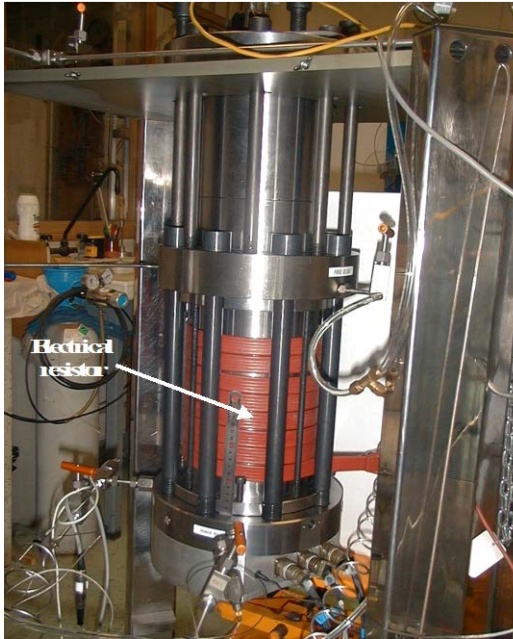
Figure 2: Triaxial cell with electrical heater developed by UJF
