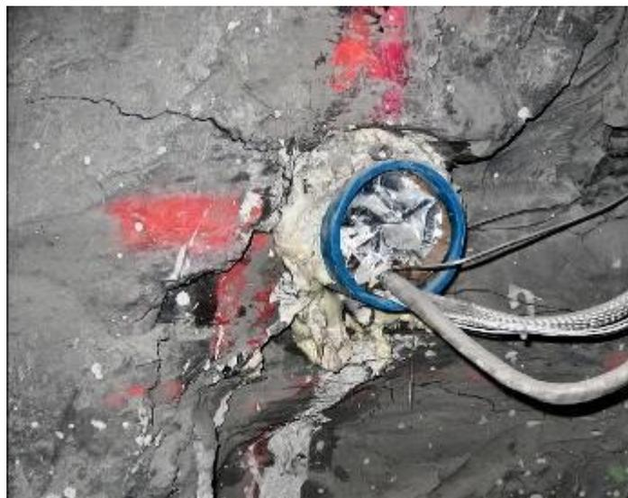
**Figure 6.44: Radial fractures occurred around the heater borehole on the GEX drift wall**
