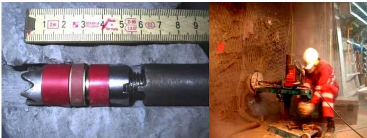
**Figure 6.16: Pore pressure and temperature sensors in slim holes (TER1401 to TER1405) as in Mont Terri HE-D experiment**
