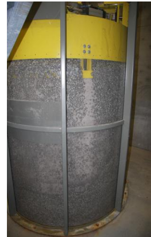
Figure 4-22. Filling of pellets into the gap between the buffer and the test hole wall.
