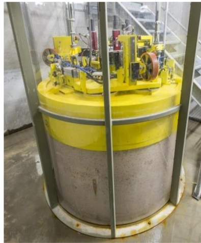
Figure 4-21. Gripper and concrete block have been lowered to the bottom of the test hole.
