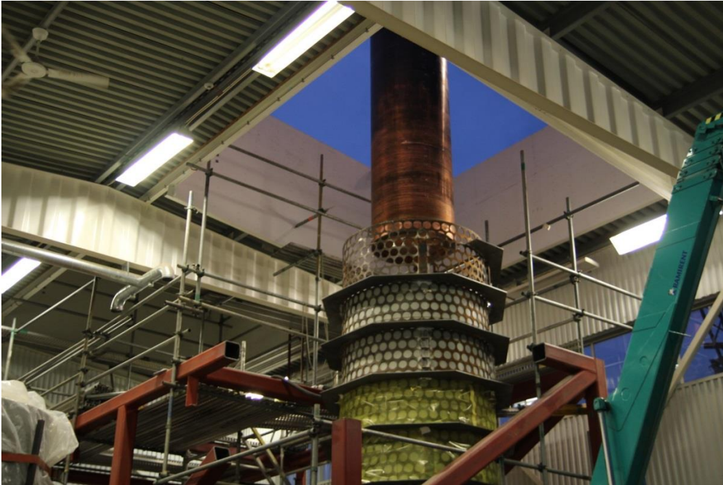
Figure 4-13. Canister being lowered into the Supercontainer during assembly. Stiffening plates for straightening the shell can be seen on its outer periphery.
