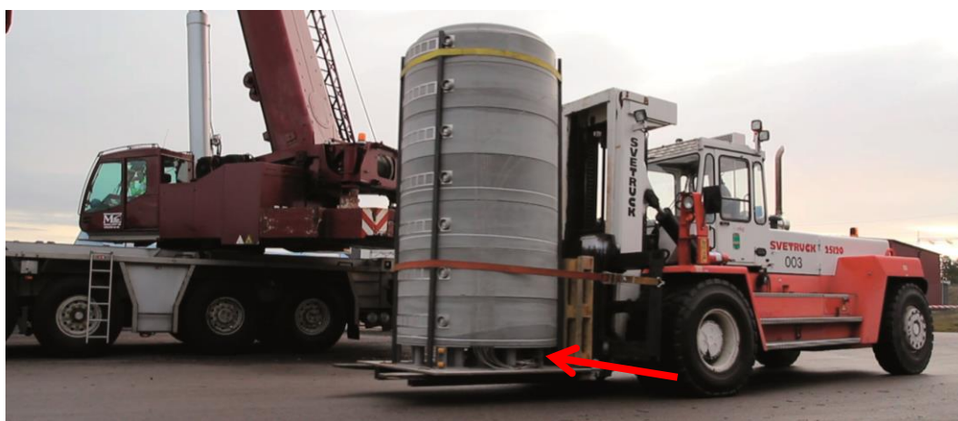
Figure 4-12. Test distance block being moved out from the assembly facility complemented by a specially designed sensor arrangement, or cable block, in which sensor cabling could be placed during transport and installation, marked with a red arrow.
