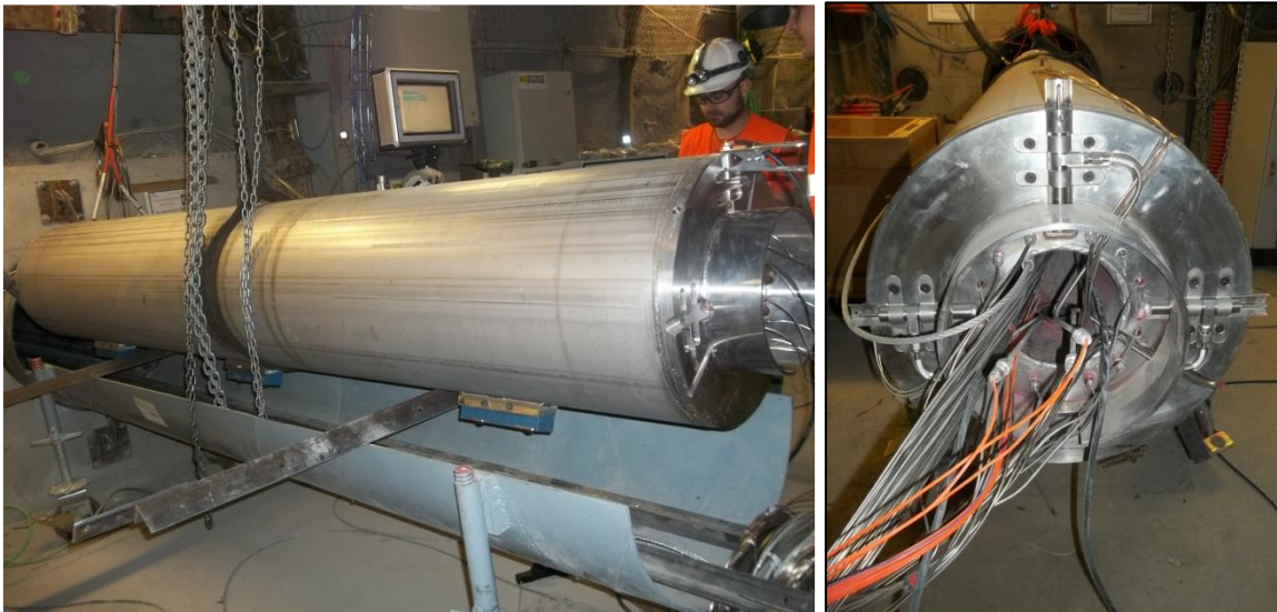
Figure 4-6. View of a heater element when it is installed (left). View of a heater/sleeve distance variation sensor section (right).
