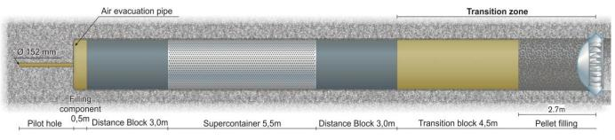
Schematic illustration of the MPT layout, the pellets filling section length has been increased from 1.3 m to 2.7 m to allow for instrumentation.
