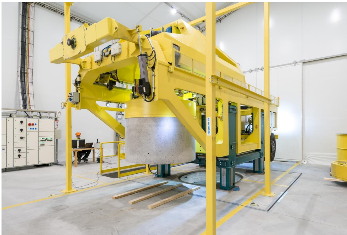
Fig. 22. Bentonite installation machine at surface level test facility.
