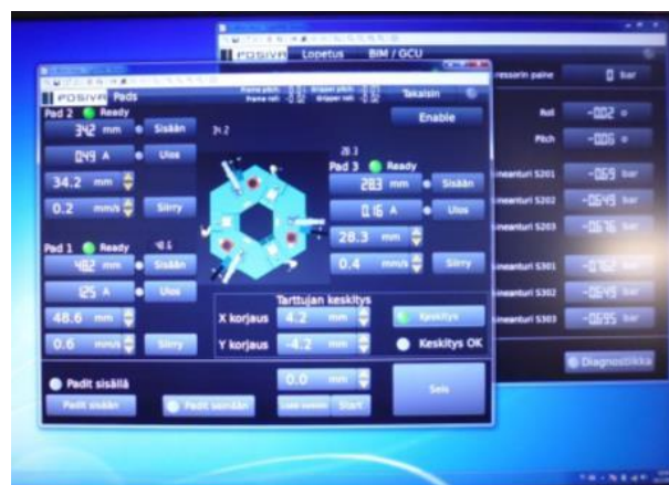
Fig. 19. Gripper control unit computer on BIM mechanical gripper
