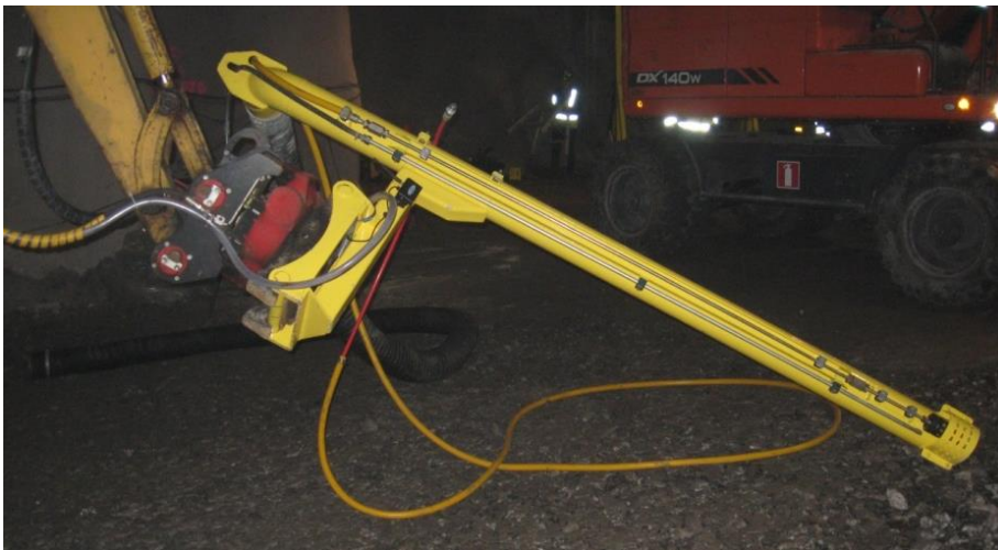
Fig. 36. Hydrodemolition device on excavator during test in ONKALO.
