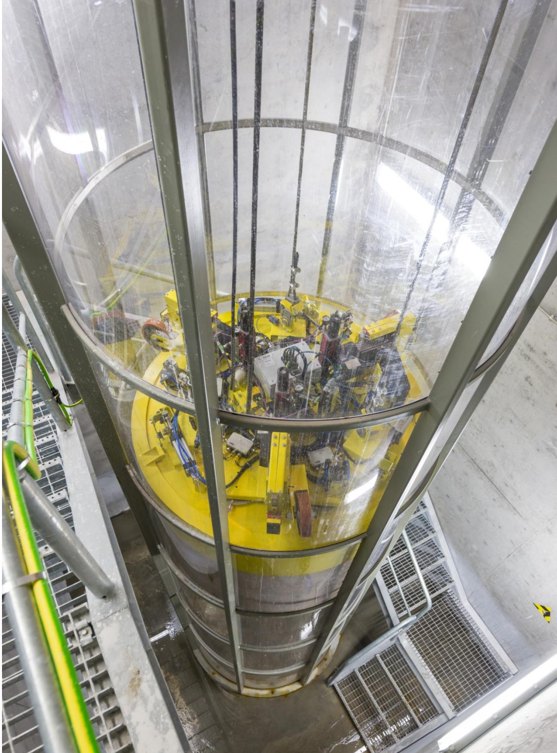
Fig. 24. Gripper and concrete block lowered into test hole.
