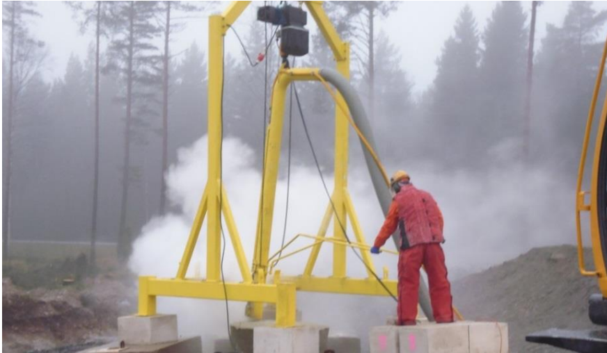
Fig. 35. Hydrodemolition device, ground level test.
