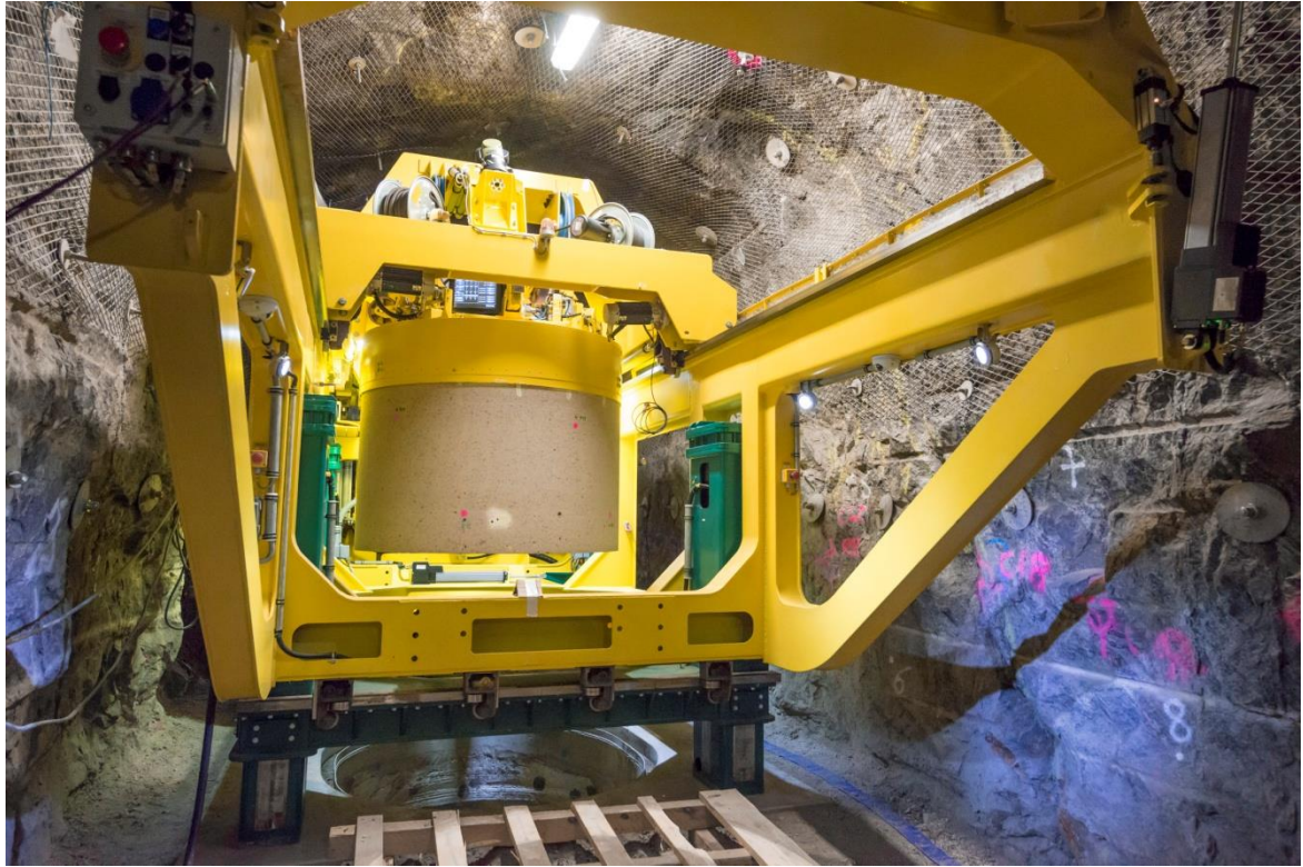
Fig. 30. Bentonite installation machine in ONKALO demonstration tunnel 1.
