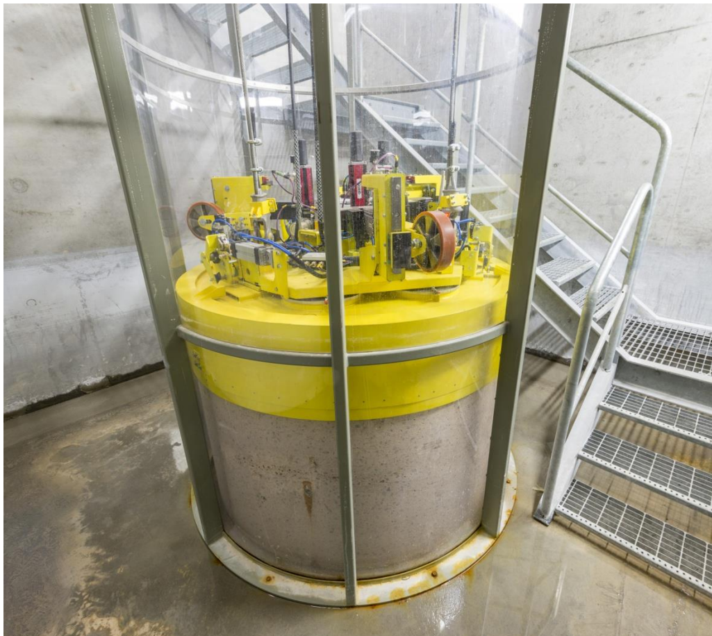
Fig. 23. Gripper and concrete block lowered into test hole.
