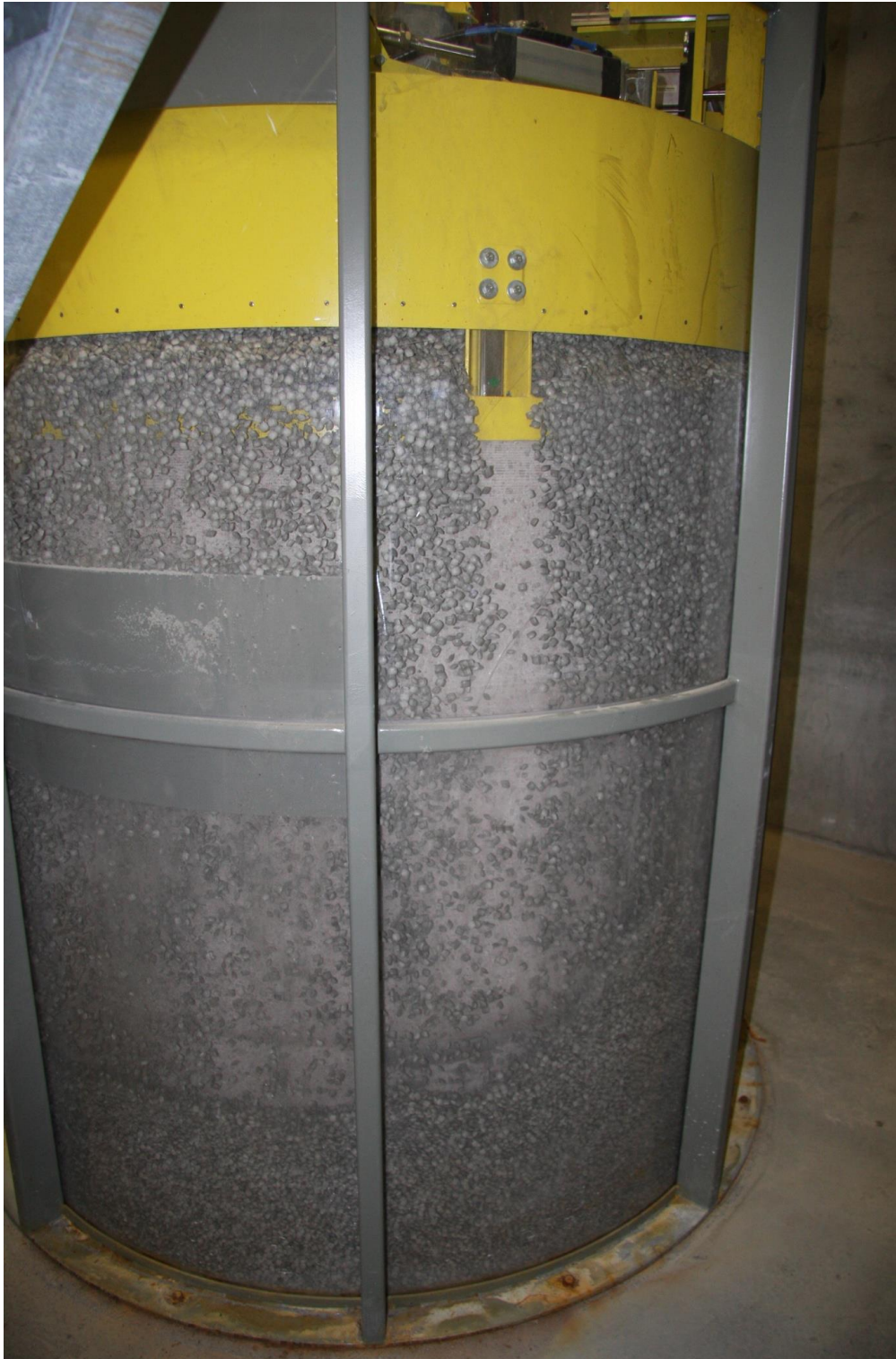
Fig. 26. Releasing of pellet into the gap between buffer and test hole wall
