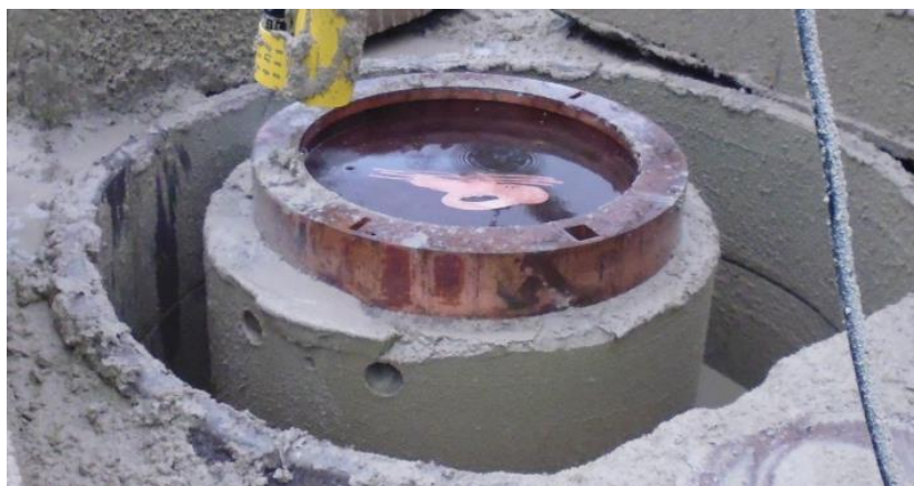
Fig. 35. Top of copper canister subjected to extended direct contact with water jet, showing polishing.
