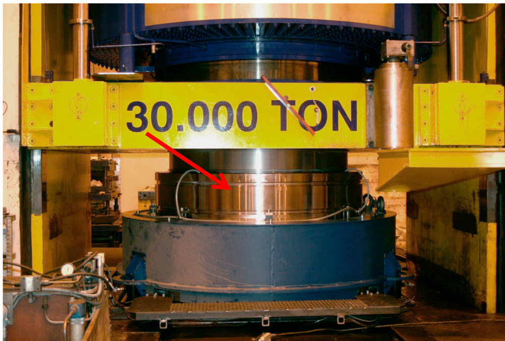
Figure 2. uni-axial compaction, the red arrow marks the mould filled with clay and ready for compaction.
