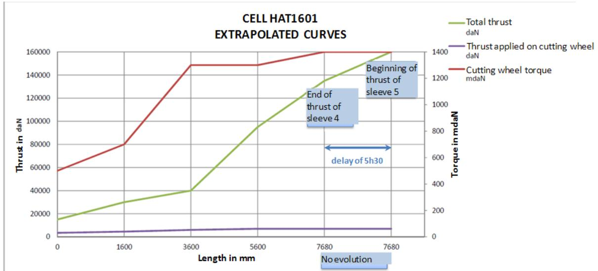
Figure 5 Changes in the various forces applied as a function of excavation progress
