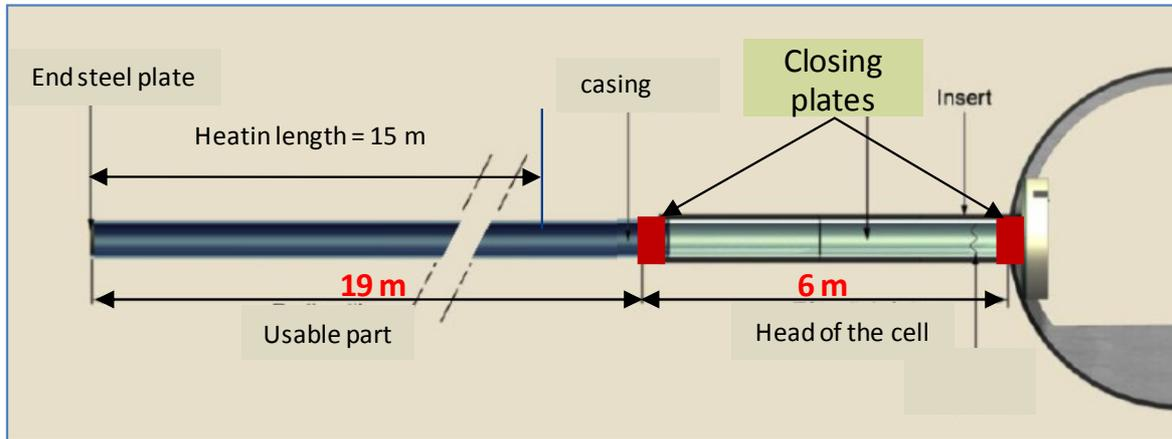
Figure 10 Dimensions of the cell for Phase 3 of the “HLW cells” Programme Unit
