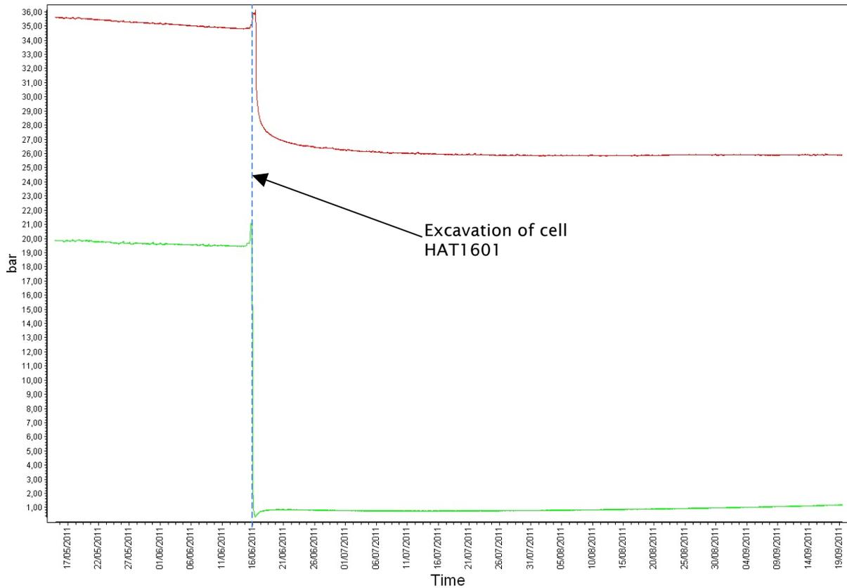
**Figure 6** Influence of cell HAT1601 excavation on the interstitial pressure in borehole ALC1615: chambers at 4.5 m from the drift (green) and 7.5 m (red)
