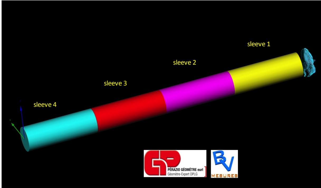
Figure 8 3D scan of the inside of the insert – sleeve section 1 is the first sleeve section driven into the rock
