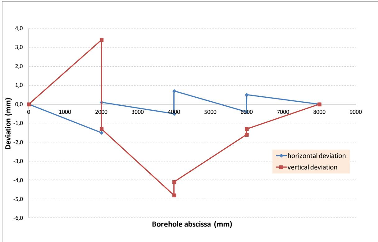
Figure 9 Horizontal and vertical deviations for each sleeve section of the insert
