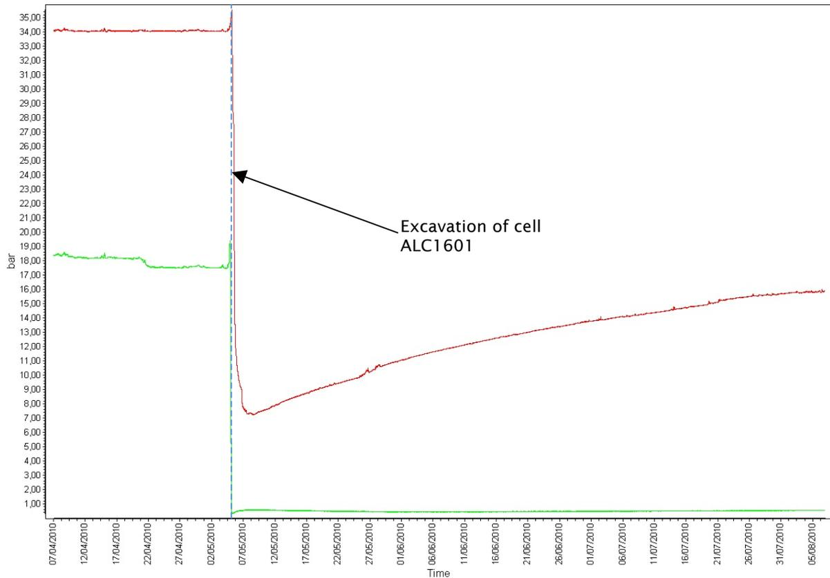
Figure 7 Influence of cell ALC1601 excavation on the interstitial pressure in borehole ALC1612: chambers at 4.5 m from the drift (green) and 7.5 m (red)
