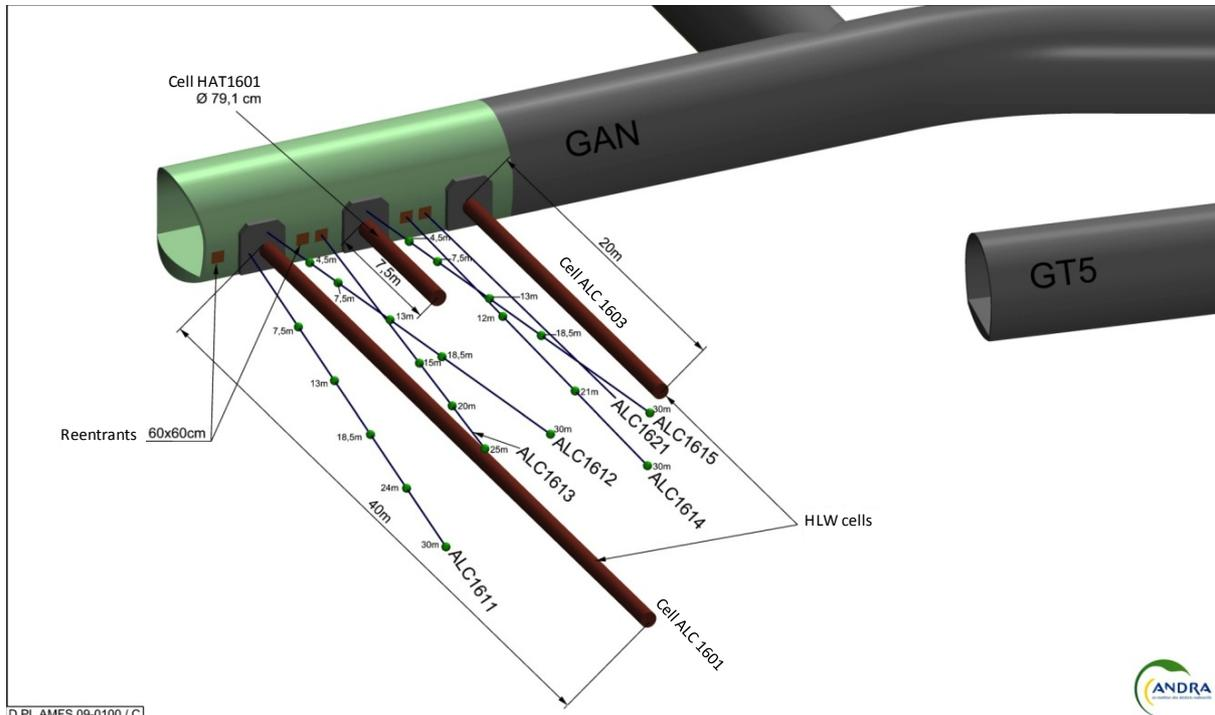
Figure 2 Position of cell HAT1601 and the peripheral boreholes
