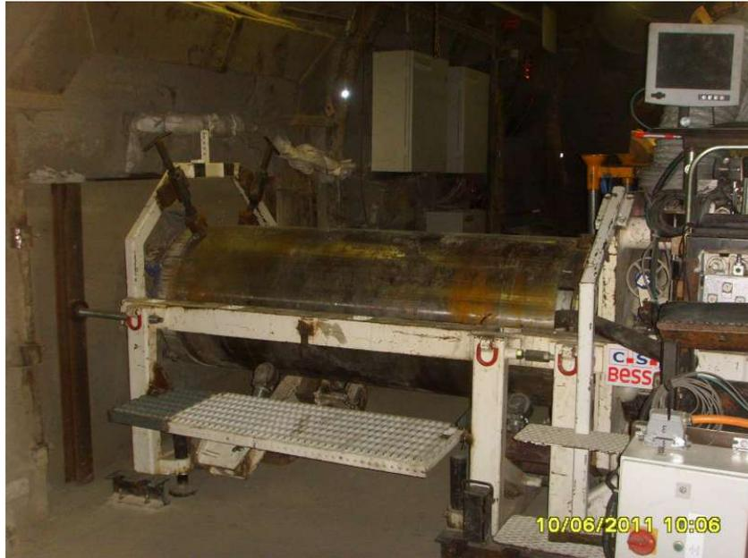
Figure 3 *Sleeve section 1 positioned on the driving station*
