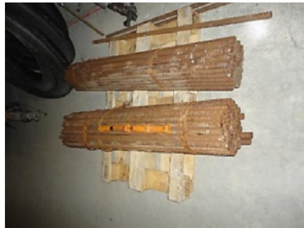
Fig. 29a: Rock bolts IBO R-32s of 7.5 m (5 x 1.5 m)
