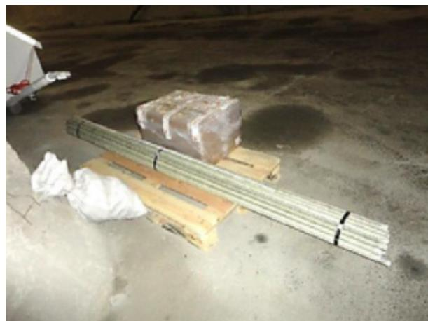
Fig. 28a: Rock bolts GFK K60-25, 2.5 m
