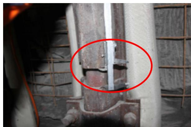
Fig. 44: Measure of the space balance with a caliper
