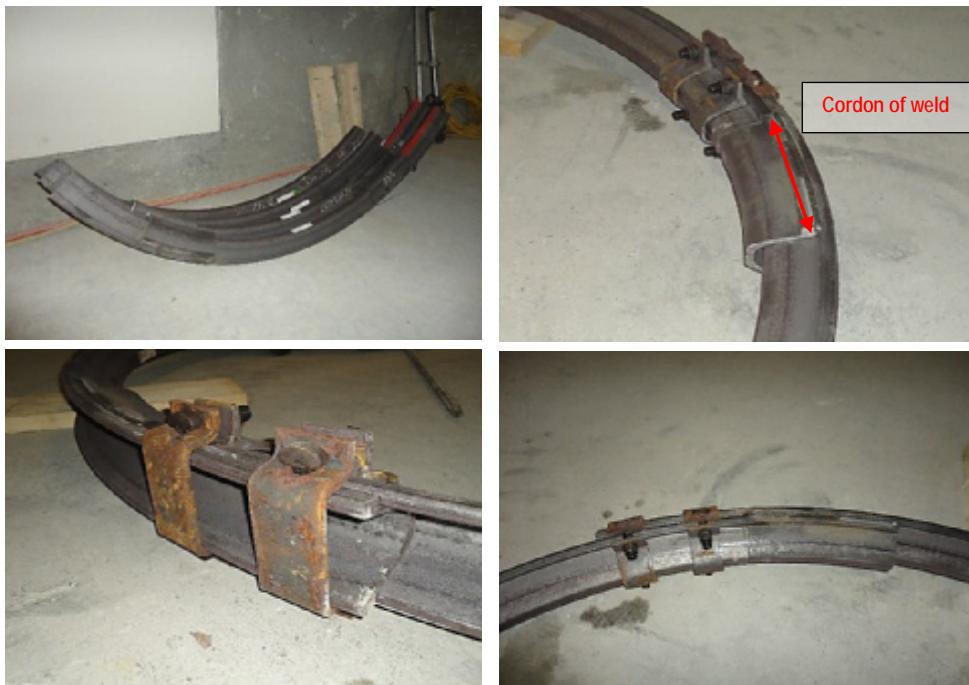
Fig. 19: TH 25 arches and splice bars
