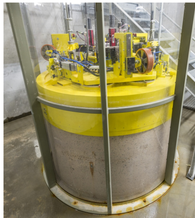
Figure 21. Gripper and concrete block has lowered into the bottom of test hole
