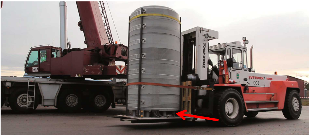
Figure 12. Test distance block being moved out from the assembly facility complemented by a specially designed sensor arrangement, or cable block, in which sensor cabling could be placed during transport and installation, marked with a red arrow
