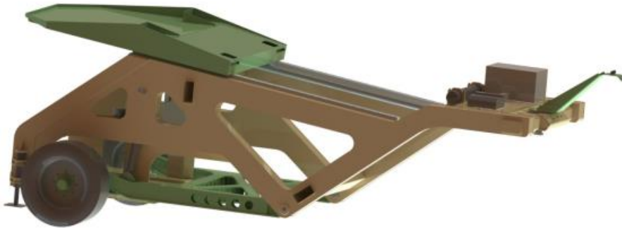
Figure 19. 3D-model of bentonite transfer device (BTD)
