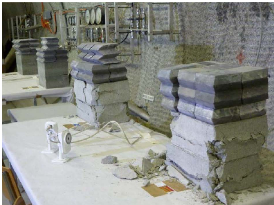
Figure 1: NAGRA - FE - Test of pedestal blocks compressive strength
