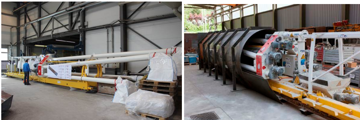
Figure 3: NAGRA - FE - Commissioning of bentonite backfilling machine at Wirtech factory
