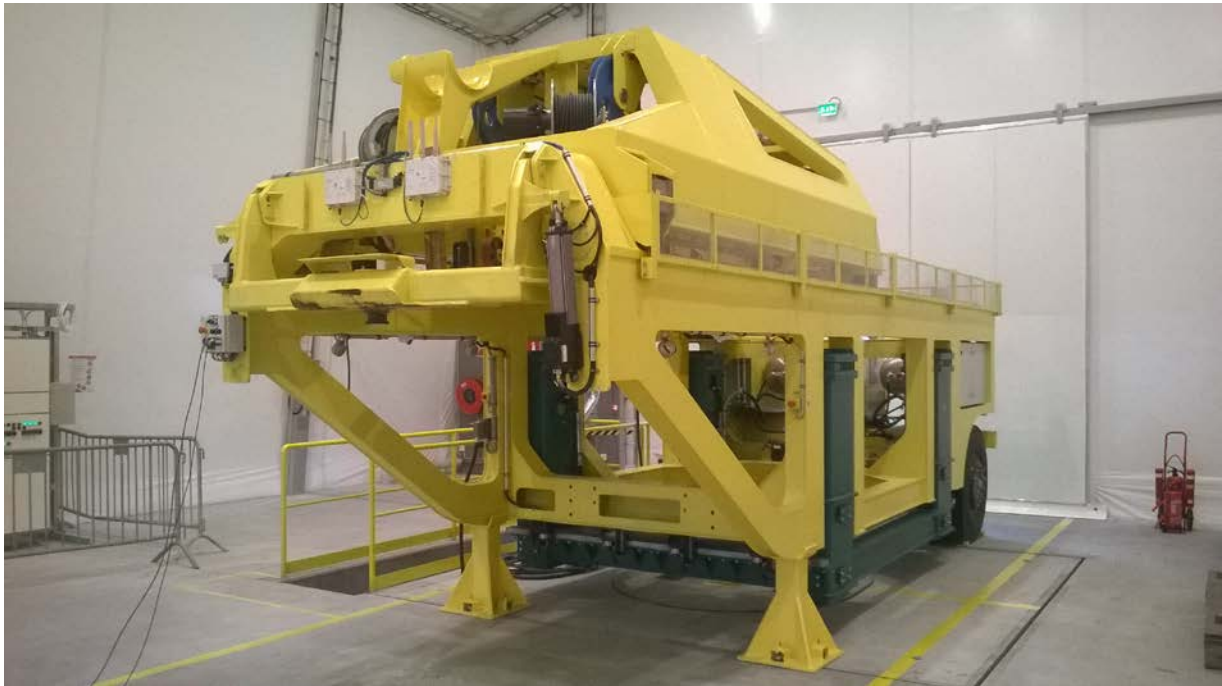
Figure 5: POSIVA - BIM machine pre-positioned above the deposition hole (mock-up)
