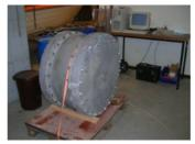
Completed installation of radial water uptake test. DAWE-concept.
