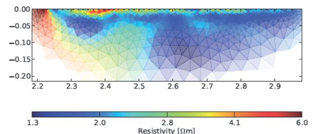
Figure 6. Electrical resistivities derived from geoelectrical measurements in the bentonite. Y-axis: depth of penetration (m).
