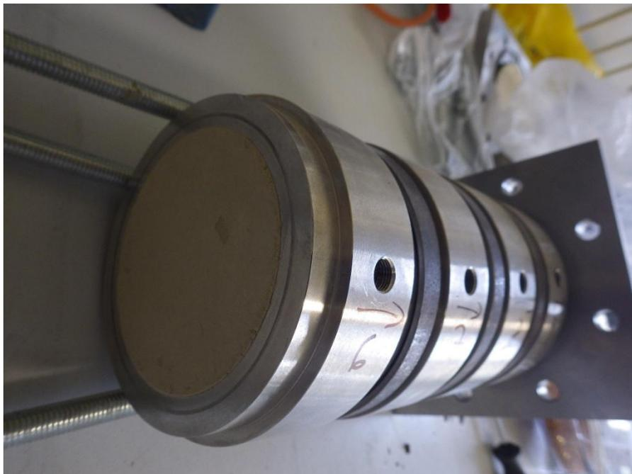
Fig. 6 The dismantling of the physical hydraulic model into individual cells.
