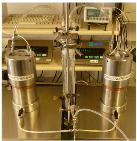
Fig. 4.19 Setup of the small-scale borehole sealing tests in steel cylinders with compacted blocks of claystone-bentonite and bentonite-sand mixtures The realistic hydraulic conditions to be expected in the drift plug/seal systems were simulated for both parallel seal samples in the following sequence:
