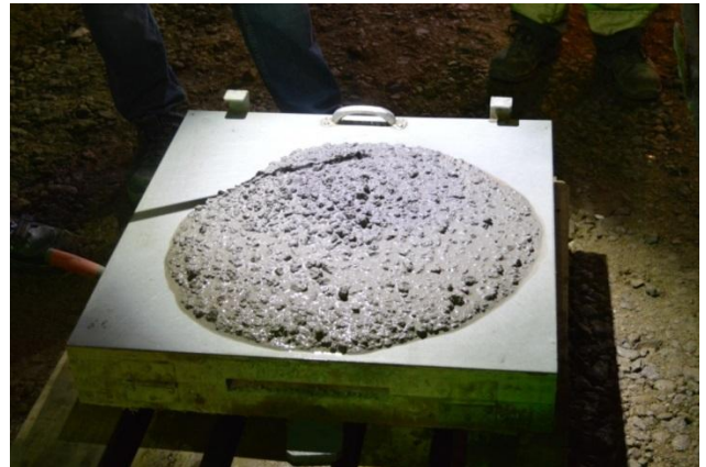
Figure 3. Quality control testing of the plug (left =cubes for quality control, right= slump flow test).
