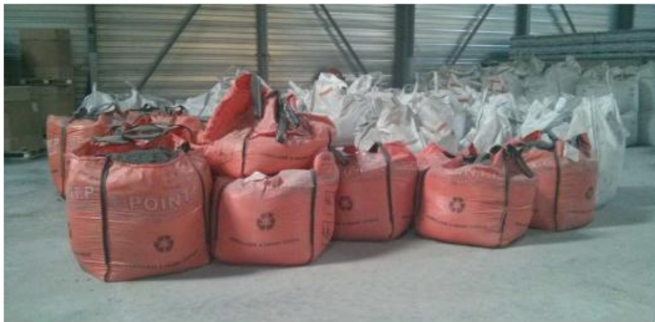
Figure 4.5: Shotcrete rebound storage in the waiting for evacuation.
