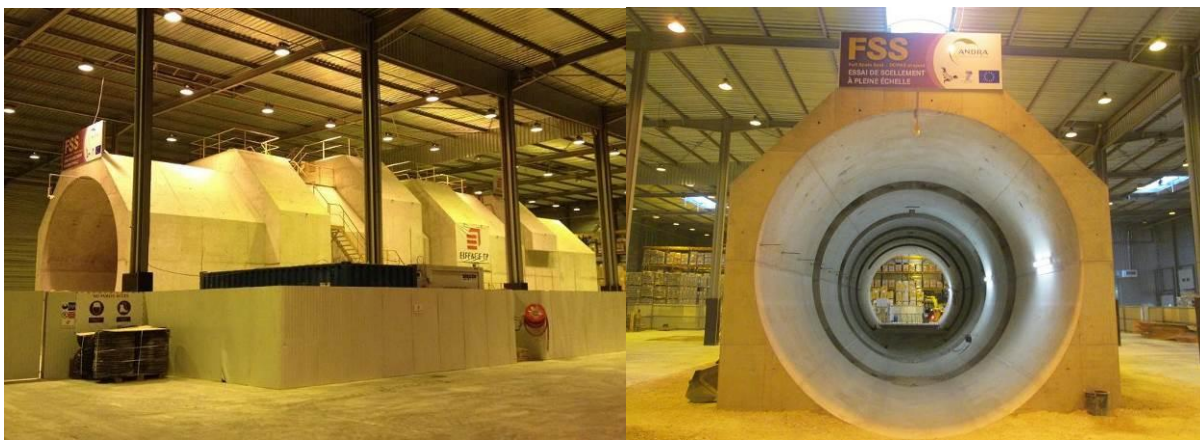
Figure 2.4: The FSS test box ready for seal construction
